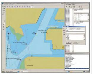
ENCEdit is a new HYPACK<sup>®</sup> module that allows you to create, modify and verify ENC data in S-57 format. ENCEdit provides you with tools to re-attribute, create, move or delete existing features. You can also create new features by manually entering coordinates, by importing data from DXF/DGN, or by transferring targets in real time from SURVEY directly into ENCEdit.
