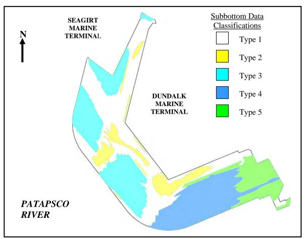
Figure 8: Overview of subbottom data classification types identified throughout the project site.
