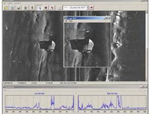
Side Scan Sonar (SSS) Support: HYPACK<sup>®</sup> provides support of SSS systems in its basic package. All analog and several digital side scan systems can be utilized with the SIDE SCAN SURVEY program. Users can display the real time data and perform targeting in real time or post-processing. A program that generates side scan mosaics in Geo-TIF format allows you to plot your results in HYPACK<sup>®</sup> or export them to your GIS.
