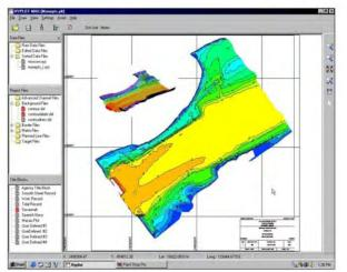
FINAL PRODUCTS: The ability to create the final products you need separates HYPACK<sup>®</sup> from the rest. The plotting program generates professional smooth sheets with soundings, grids, graphics and contours in a WYSIWYG display. The VOLUMES program is the de facto standard of the U.S. Army Corps of Engineers for the computation of quantities in dredging projects. TIN MODEL creates surface models that can be used for contouring, volume computations and surface visualization.
