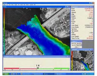
SURVEY: HYPACK<sup>®</sup> contains interface drivers to over 200 devices includings positioning systems, echosounders, heave-pitch-roll sensors, gyros and other types of equipment. SURVEY supports a single vessel or multiple vessels, along with towfish and ROVs. Data is logged with incredible precision (<1mSec). Survey data and windows can be broadcast over a network to any other computer or saved to a file using our Shared Memory Output routines.
