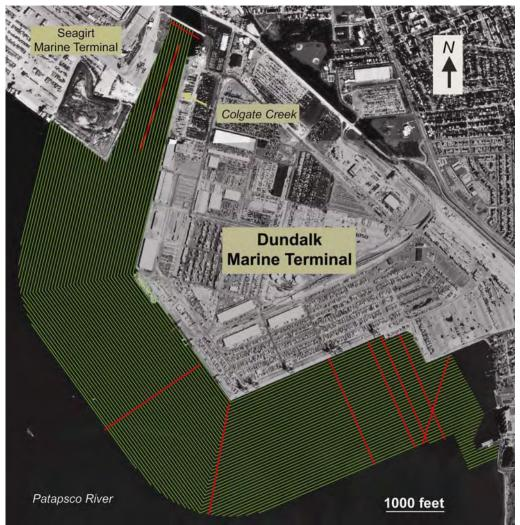
Figure 2: Location map showing the planned Task 1 and 2 survey lines (green) and pre-defined CH2M sampling transects (red).
