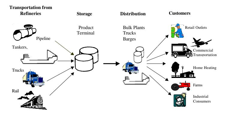
Pipelines, vessels, trucks and rail cars are the four methods of oil transport used in insuring that movement from one facility to another can continually occur (Figure 3). Most of the time, this movement of oil occurs without incident. However, this distribution network is not perfect. Spills, some small with little or no consequences and some large that can result in long term interruption of lifestyle for those affected, happen.
