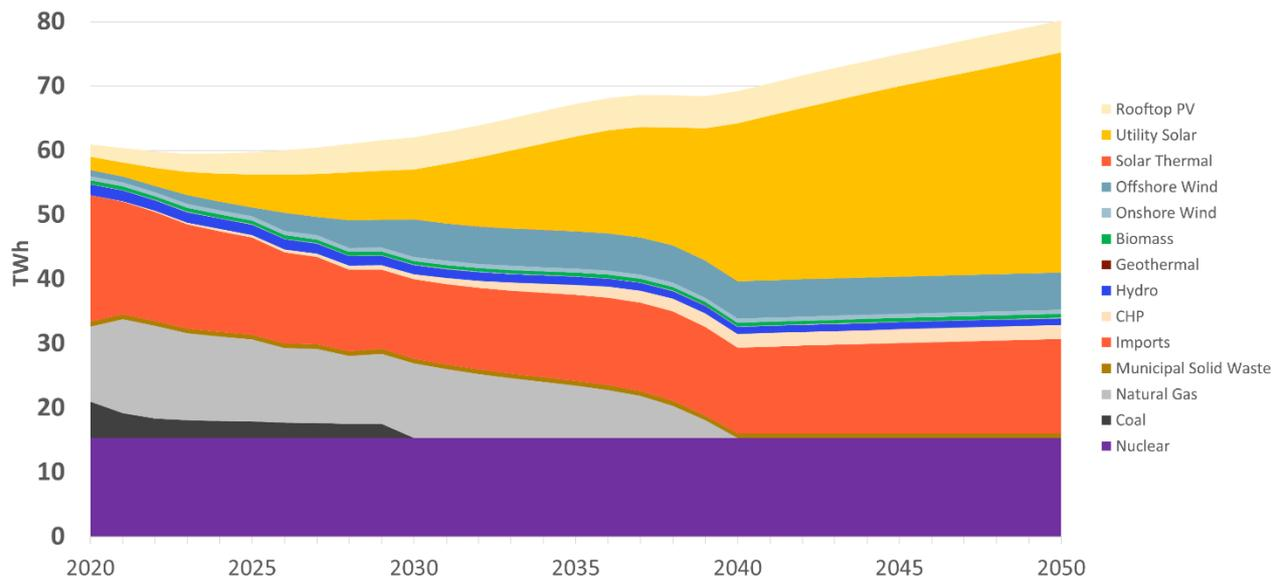
**Figure 3.1-1. Maryland electricity mix through 2050 in the 2030 GGRA Plan.** Fossil power plants without carbon capture and storage technology (gray colors) are eliminated by 2040 and replaced with clean and renewable energy. “Imports” reflects electricity generated outside of Maryland but consumed in Maryland. Analysis assumes no carbon capture or new nuclear facilities available before 2030.
