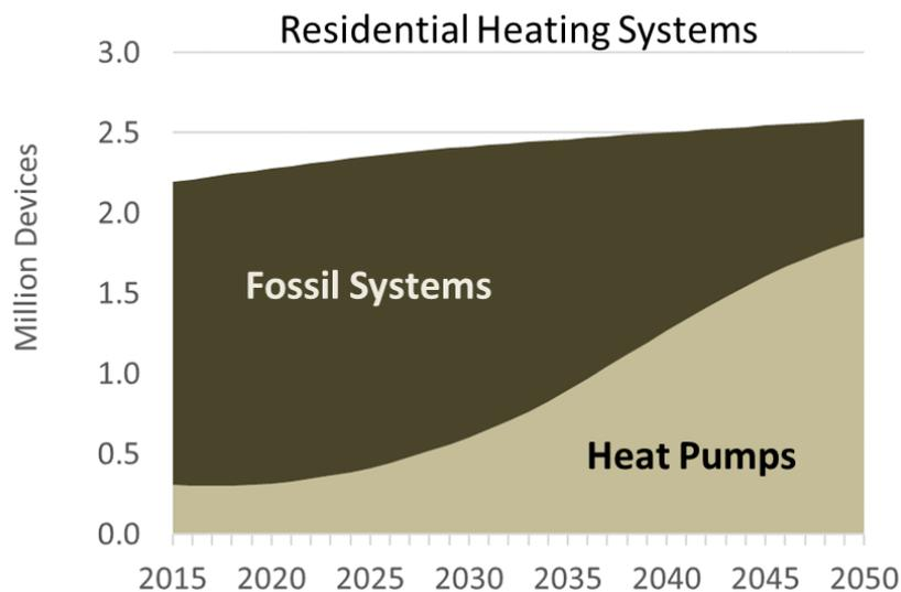
**Figure ES-14. Composition of residential heating systems in Maryland in the 2030 GGRA Plan.** Thanks to incentives for heat pumps, increasingly large shares of fossil systems are replaced by heat pumps when they reach the end of their useful life. Heat pump use in commercial buildings projected to be lower.
