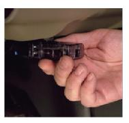
The VEIP facility's Customer Service Representative will plug the device into the eligible vehicle's OBD data link connector. After reading the vehicle's OBD data and comparing the data to the programmed VEIP readiness criteria, the device will:
