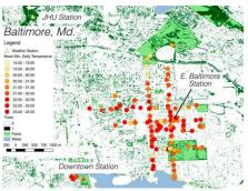
Fig. 3. Locations of the 135 sensors in eastern Baltimore. The color scale shows \(\overline{T}\), the temporal mean of daily minimum temperatures for 1 Jun-15 Sep 2015.
