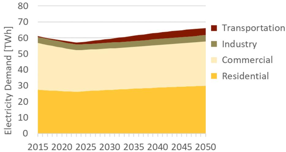
Figure 3-10. Total Electric Load by Sector, Reference Scenario
