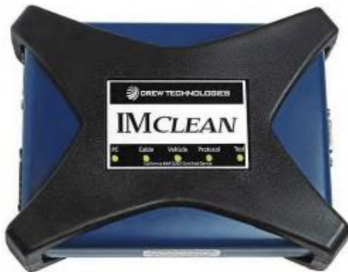
Figure 2: Opus IVS IMclean-04 Data Acquisition Device (DAD)
