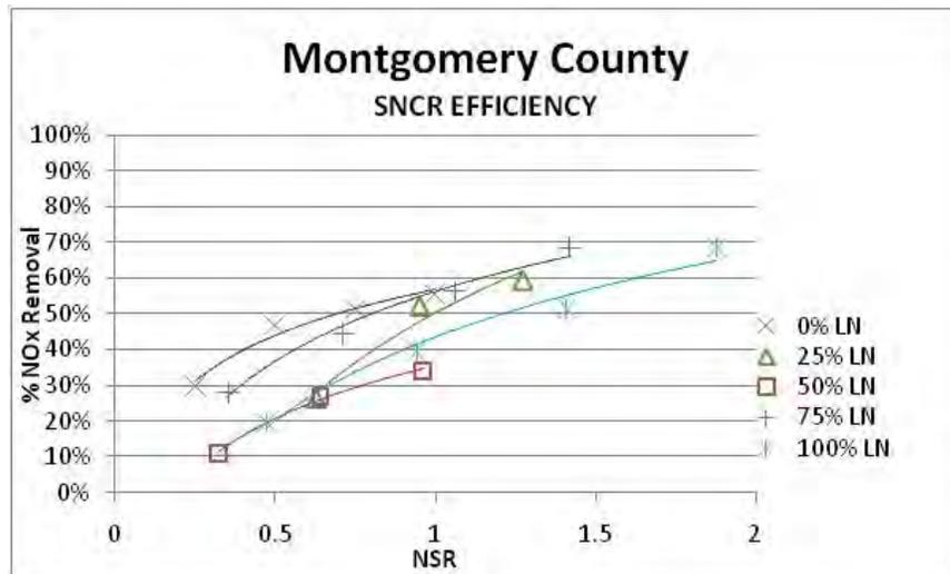
**Figure 8. SNCR Efficiency at Various LN™ Settings**
