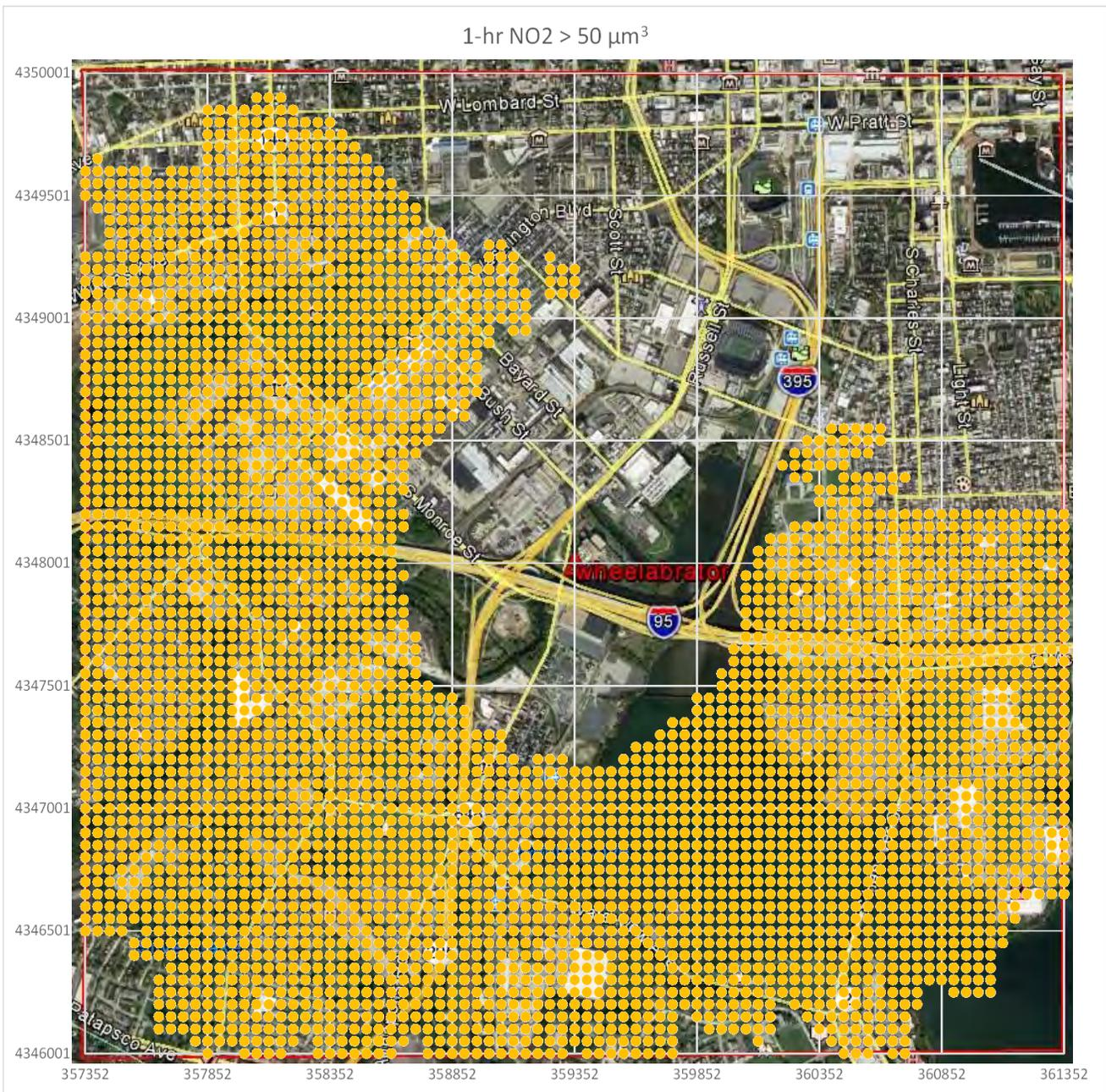
**Figure A.6. Fine grid: modeled max 1-hr-NO<sub>2</sub> concentrations exceeding 50 μg/m<sup>3</sup>**
