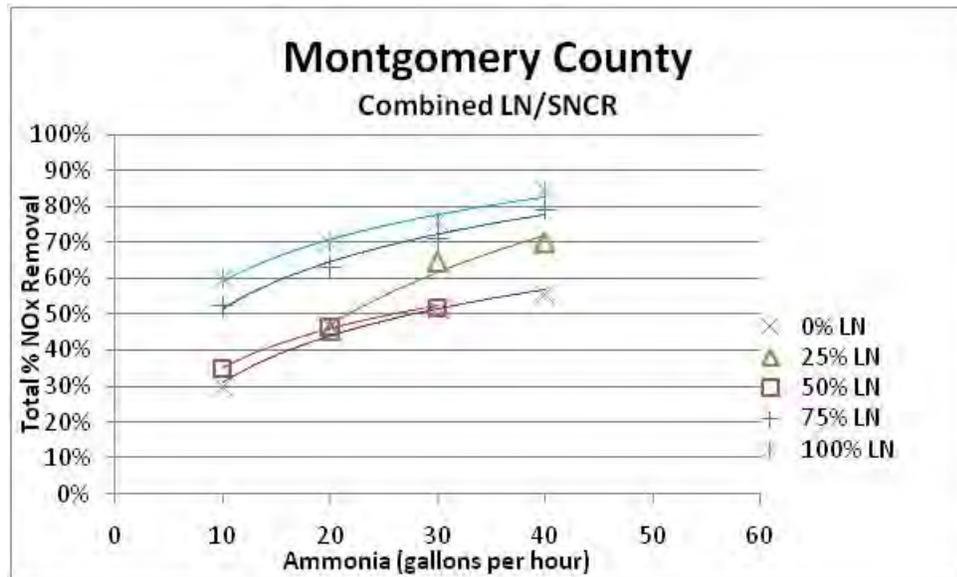
Figure 11. Combined Performance LN<sup>TM</sup>/SNCR - Consumption
