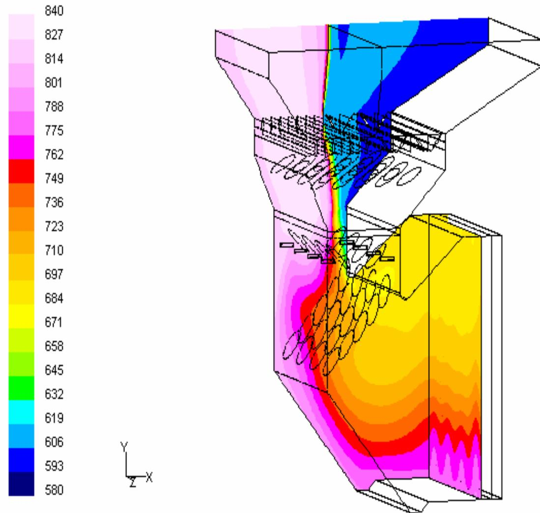
Exelon Handley 3 SCR @ MCR: Ammonia Mixers Away from Walls. Inlet & Outlet Crossmixer Stages, Geo 7
