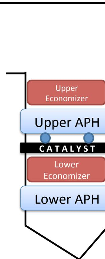
One or several layers of catalyst installed in-duct; each 2-3 meters thickness
