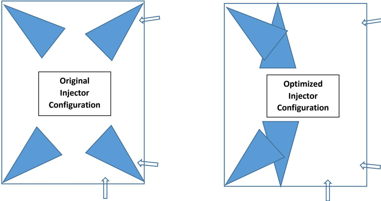
With the as-found original injector configuration using 4 corner urea injectors, NO<sub>x</sub> averaged around 175 ppm, NO<sub>x</sub> removal ranged from 14-21% with urea utilization around 25%. This configuration was sufficient to maintain compliance the PSD permit equivalent limit of about 185 ppm.
