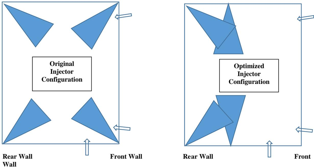
With the as-found original injector configuration using 4 injectors located in furnace corners, NO<sub>x</sub> averaged around 175 ppm while NO<sub>x</sub> removal ranged from 14-21% with urea utilization
