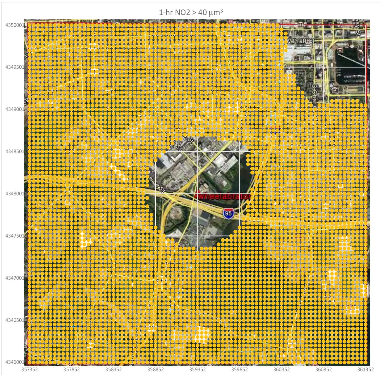
**Figure A.3 Fine grid: modeled max 1-hr-NO<sub>2</sub> concentrations exceeding 40 μg/m<sup>3</sup>**
