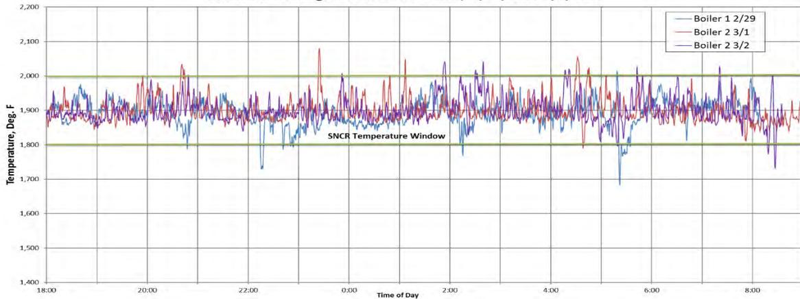
SNCR System Optimization Test Results: Optimization testing was performed by evaluating different injector configurations (number of injectors and furnace locations) and varying urea injection rates. Optimization testing found that urea injection biased more toward the rear of the furnace using the 2 rear corner and 2 rear side wall injectors, as shown in the figure below, provided the best improvement in NO<sub>x</sub> reduction and urea utilization over all other injector configurations.
