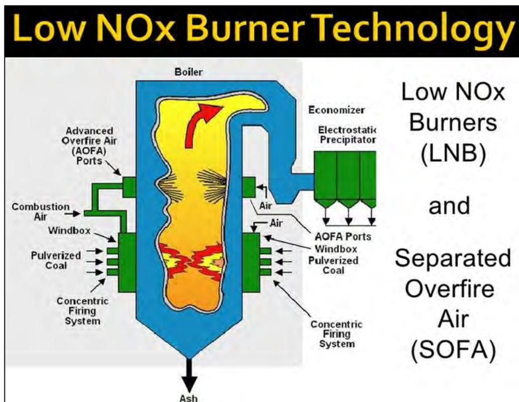
Ultra Low NO<sub>x</sub> Burner (ULNB) can achieve NO<sub>x</sub> emission levels in the order of single digits in ppm.<sup>28</sup>
