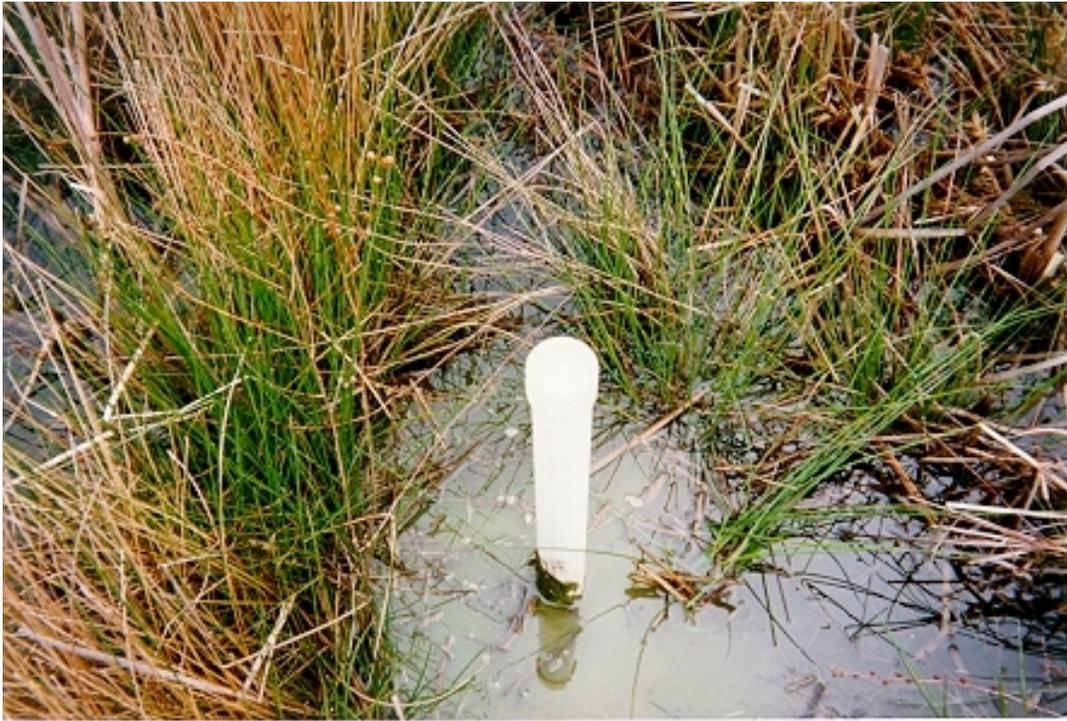
Figure 3.1: Groundwater monitoring well used before construction and also through monitoring after construction (photo Noble)
