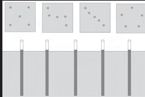
Fig. 3. Five replicate IRIS tubes should be inserted into a uniform area or "plot" that typically covers 1- to 2-m<sup>2</sup>. The tubes can be placed in any convenient arrangement that ensures their even distribution over the area of interest.
