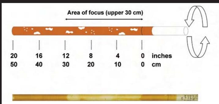
Fig. 5. Estimates of the proportion of the tube area where paint has been removed should be made while rotating the tube. When focusing on issues of hydric soils, the area of interest is the upper 30 cm (12 inches) of the soil.
