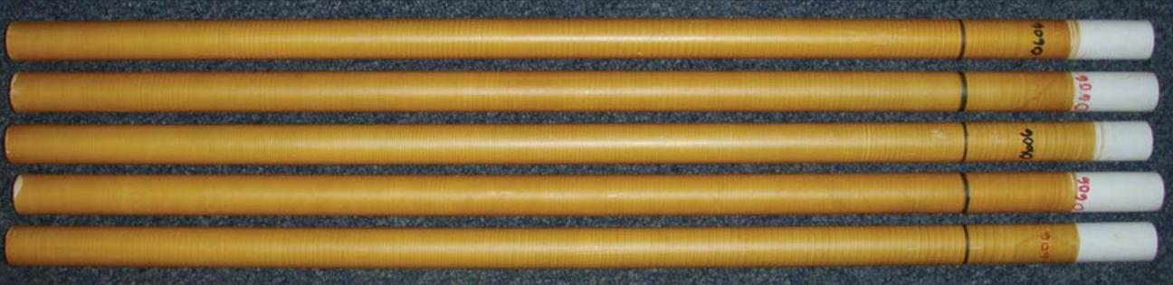
Fig. 1. Set of five IRIS tubes with line marking 50 cm (20 inches) from the bottom of the tube. The notation on the tube identifies the particular batch of paint used in making these tubes (0606).
