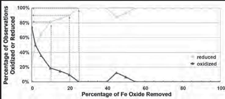
Fig. 6. The proportion of Fe oxide paint removed from a 10-cm (4-inch) section of IRIS tube related to the percentage of Eh pH observations where the soil was reduced or oxidized according to the Technical Standard of the National Technical Committee on Hydric Soils. Note that when 20% of the Fe oxide paint is removed from a 10-cm (4-inch) zone, the soil was reduced in 90% of the observations. Modified from Castenson and Rabenhorst (2006).
