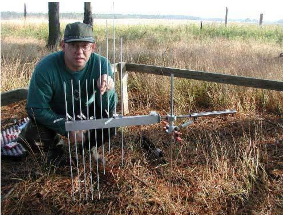
Figure 12. Reading the Rod SET at Blackwater National Wildlife Refuge. (Photo from the USGS Surface Elevation Table website at <http://www.pwrc.usgs.gov/set/readSET.html>.)
