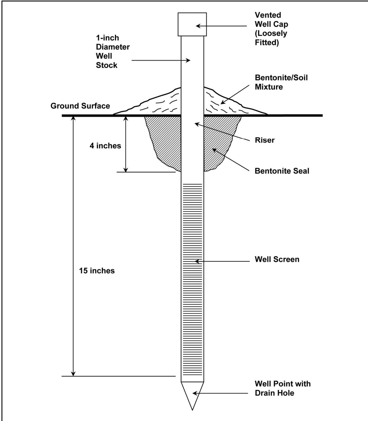
Figure 3. Standard 15-in. monitoring well installed by driving
