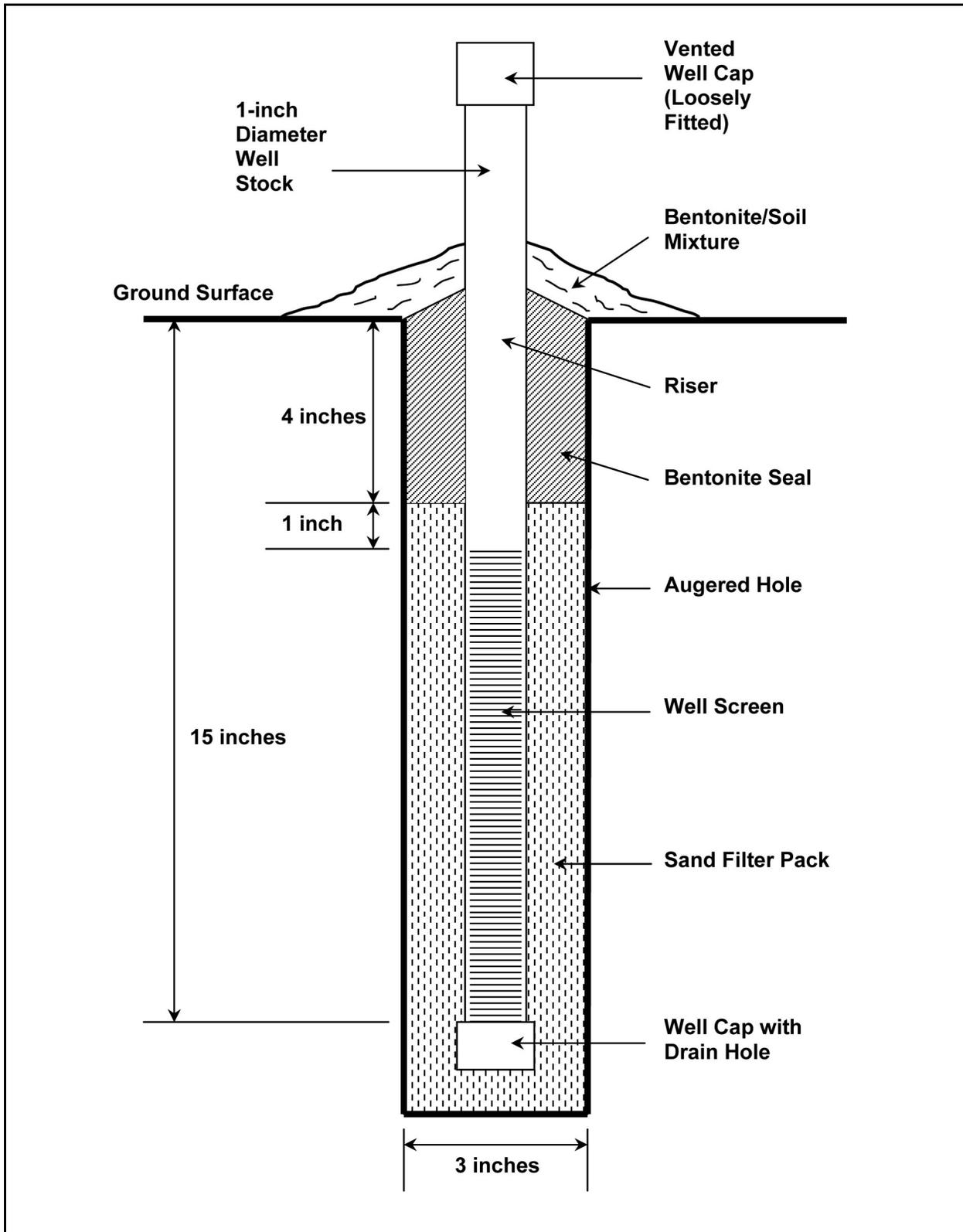
Figure 2. Standard 15-in. monitoring well installed by augering
