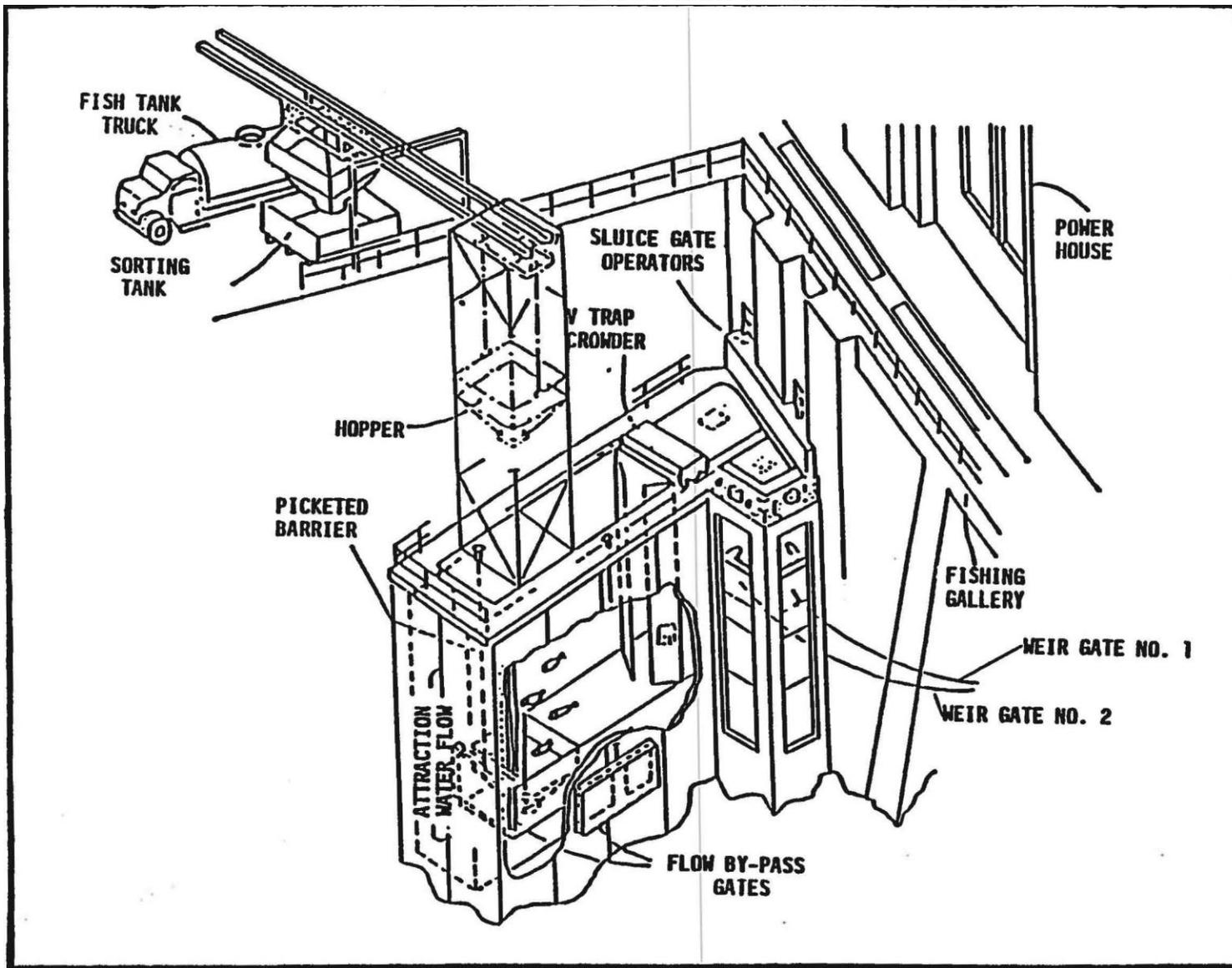
**FIGURE 5.1-2: EAST FISH LIFT SCHEMATIC DRAWING**
