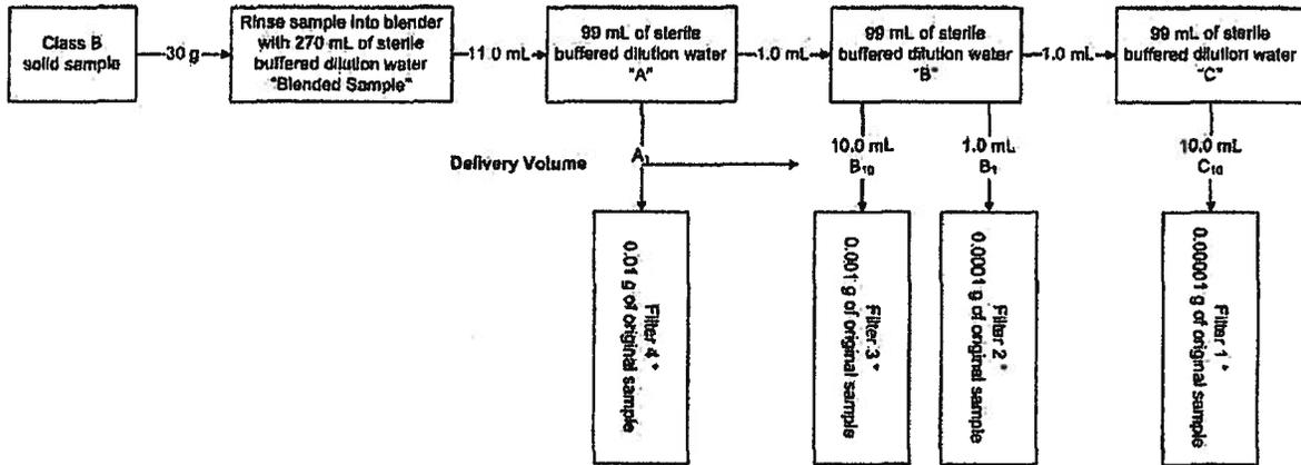
\* Samples should be filtered in order of highest dilution (least sample volume) first to avoid carry-over contamination. Filtration should take place in the following order: filter 1, 2, 3, and 4.
