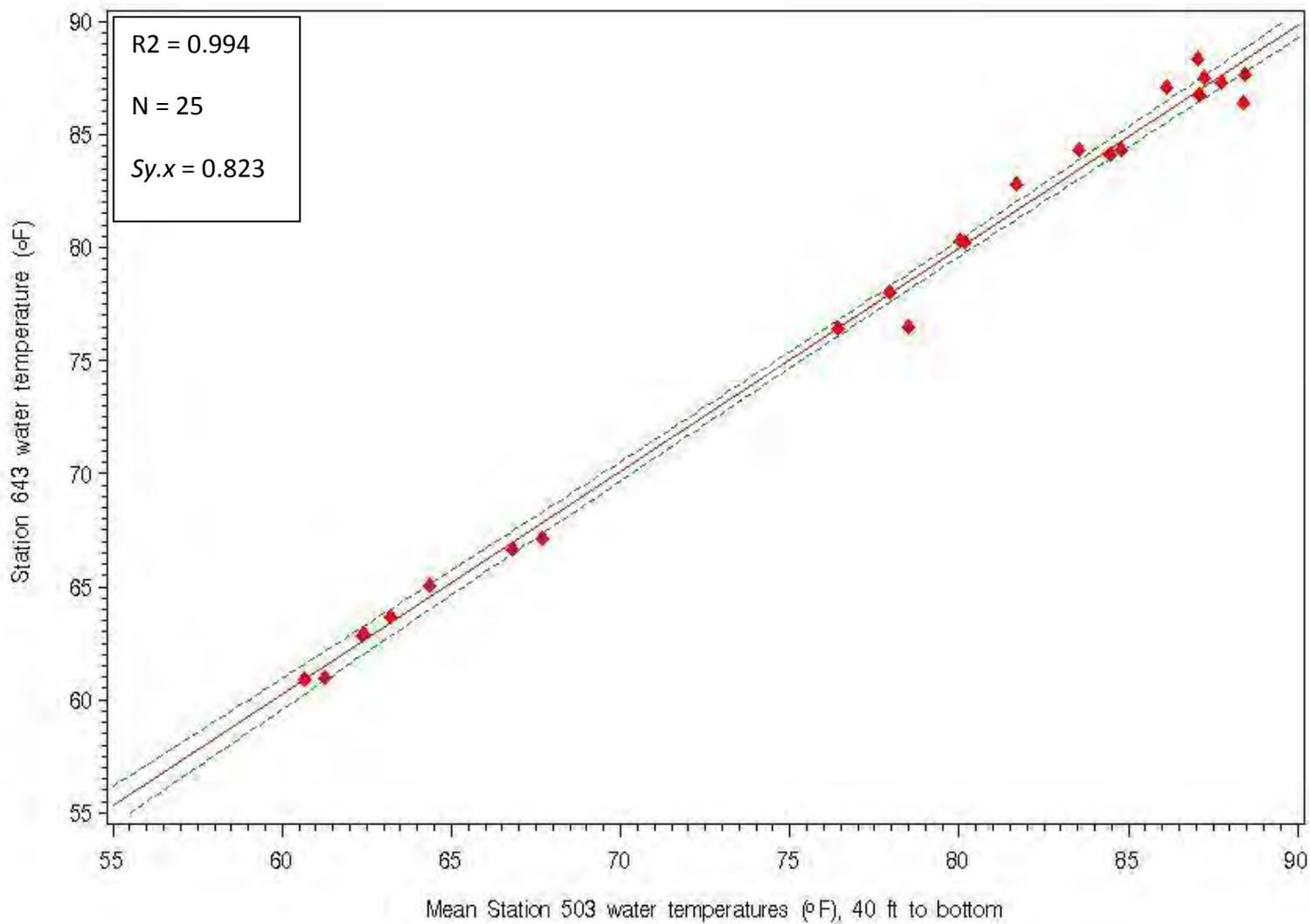
**FIGURE 4-36: COMPARISON OF PREDICTED AND OBSERVED WATER TEMPERATURES AT STATION 643. PREDICTIONS MADE FROM WATER TEMPERATURE AT  $\geq 40$  FT DEPTH STATION 502.**
