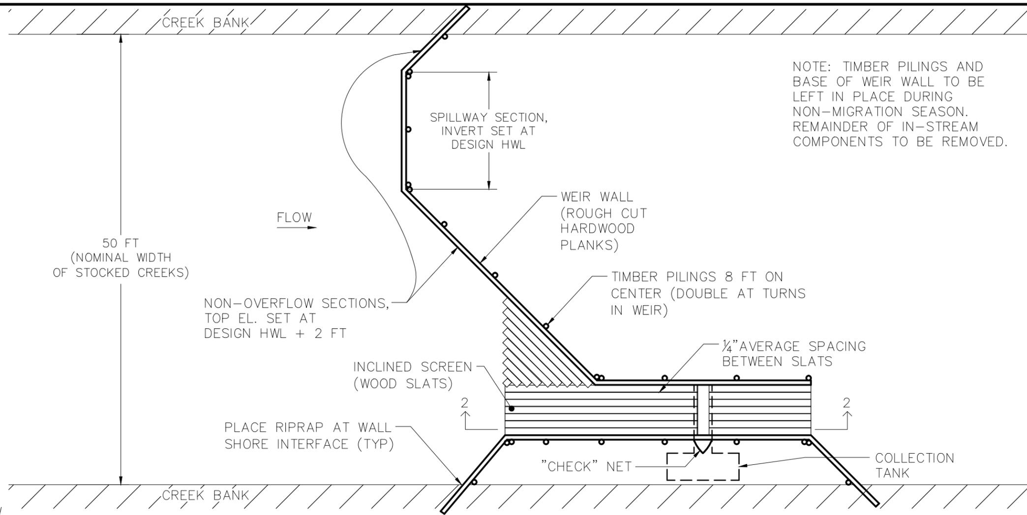
NOTE: TIMBER PILINGS AND BASE OF WEIR WALL TO BE LEFT IN PLACE DURING NON-MIGRATION SEASON. REMAINDER OF IN-STREAM COMPONENTS TO BE REMOVED.
