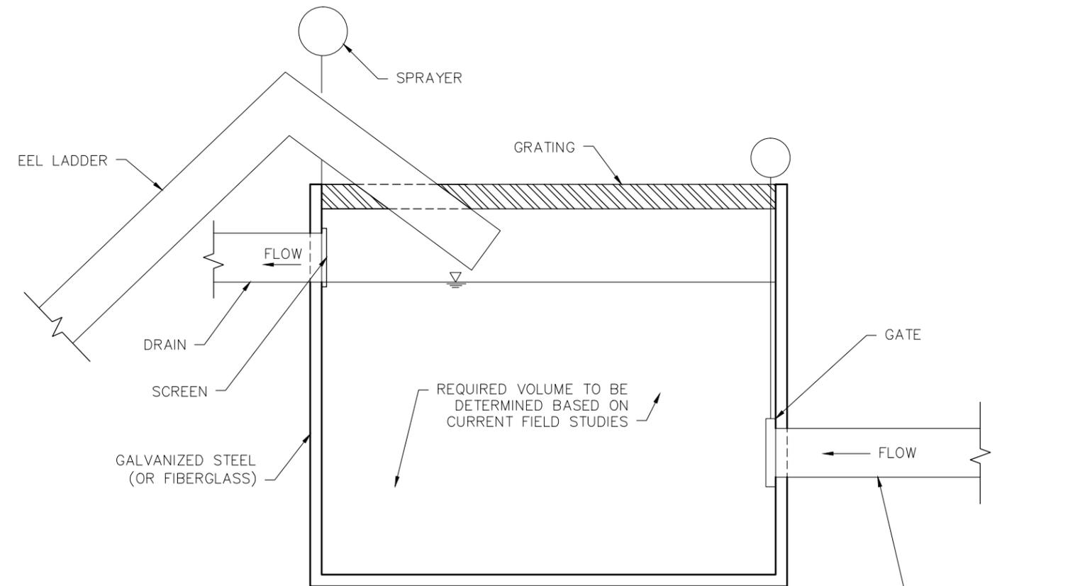
3 EEL TRANSFER TANK (PIPE THROUGH DAM)
