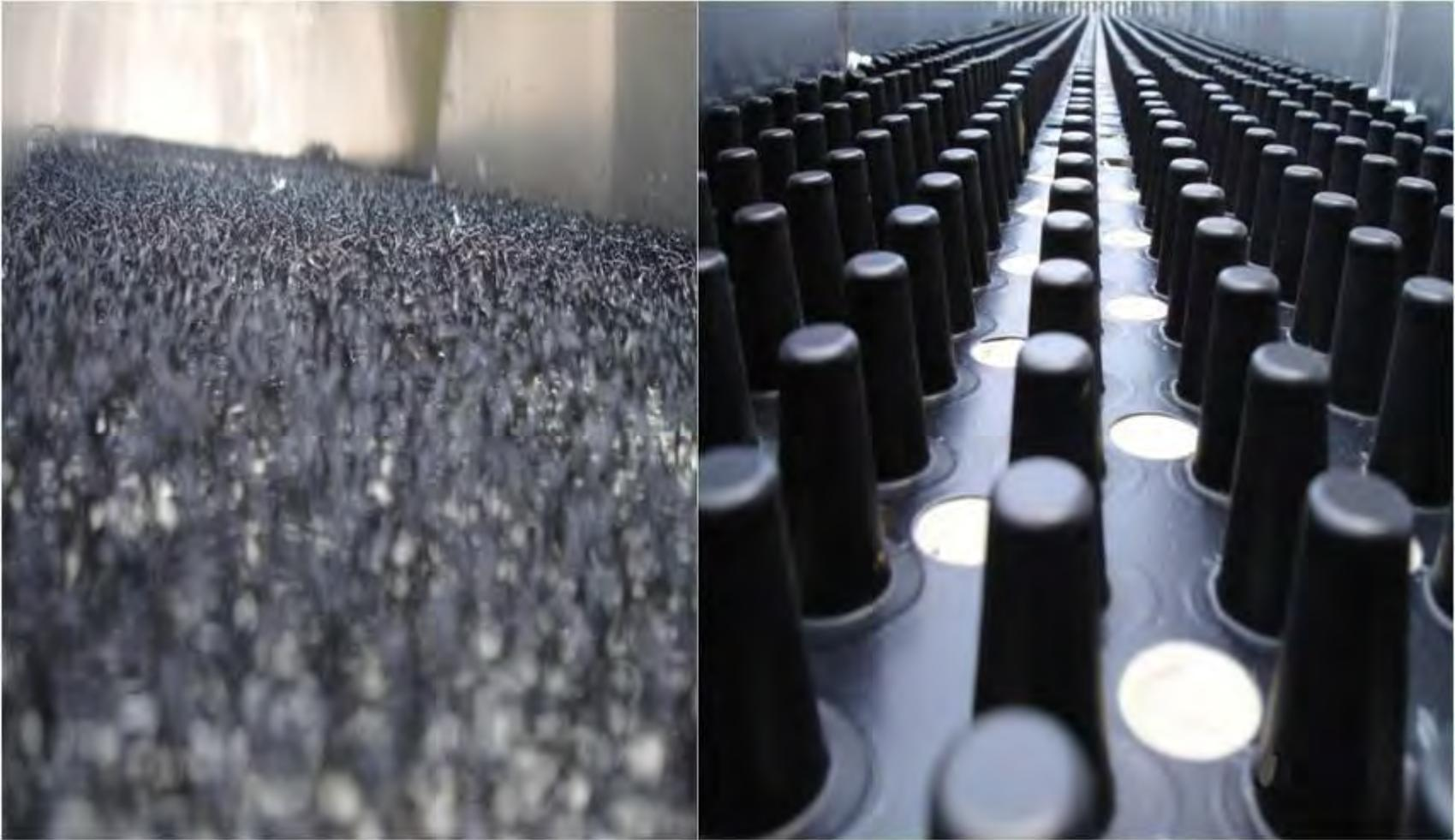
**FIGURE 4.3-1: ENKAMAT® AND AKWADRAIN™ SUBSTRATE.**
