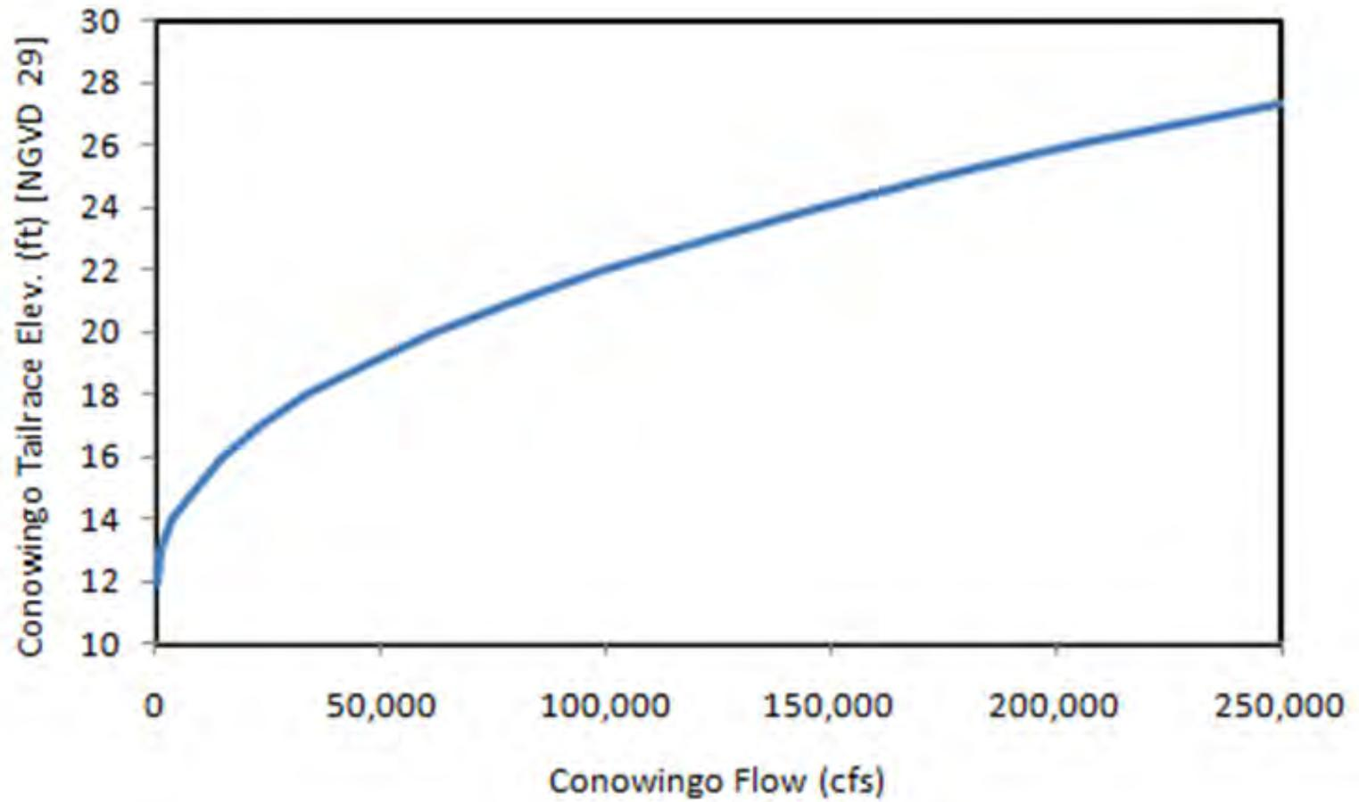
**FIGURE 2.1.4-1: TAILWATER RATING CURVE BELOW CONOWINGO DAM**
