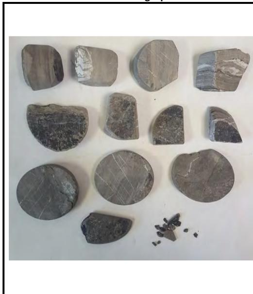
**Type II—Retained specimen consist of large and small fragments.**
