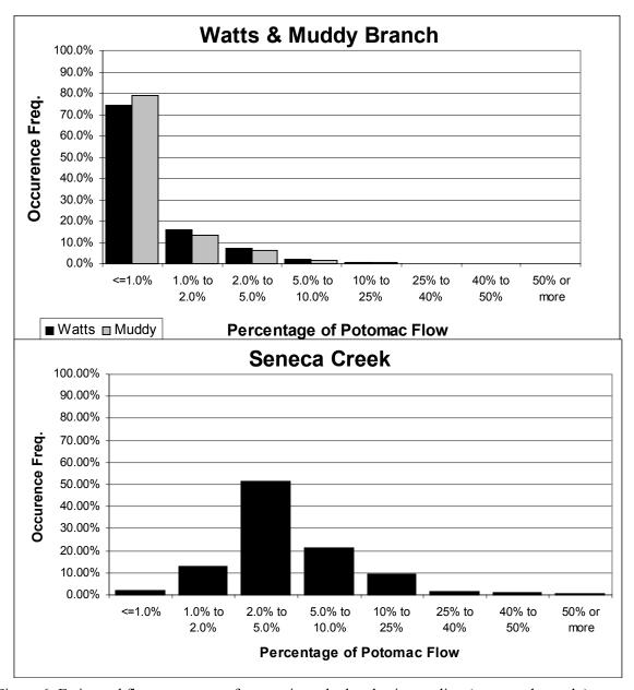
Figure 6: Estimated flow occurrence frequencies calculated using scaling (wet weather only)
