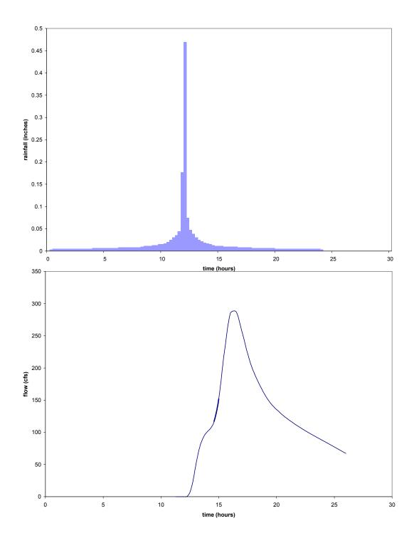
Figure 4: The hyetograph (top) and hydrograph (bottom) for the 3 times per year storm in Watts Branch
