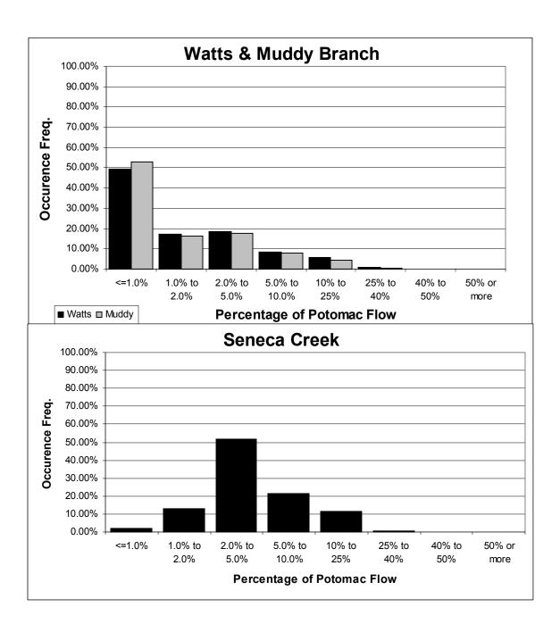
Figure 5: Estimated Flow Occurrence Frequencies calculated using the Simple Method
