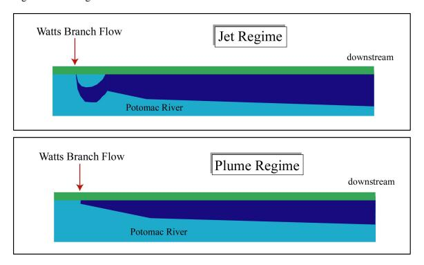
Figure 3: A schematic example of the jet and plume regimes produced by CORMIX
