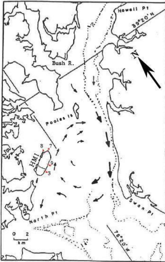
**Figure 1- 1: Schematic surface gyre circulation in the upper Chesapeake Bay and relation to HMI DMCF (modified from Wang, 1993). Red arrows indicate approximate location of the HMI DMCF spillways; numbers 3, 7, 8 and 9 identify spillways 003, 007, 008 and 009, respectively.**
