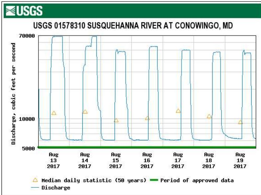
Figure 19: Graph of river discharge (cubic feet per second) at USGS gage 01578310, located immediately downstream of the Conowingo Dam at Conowingo, MD.
