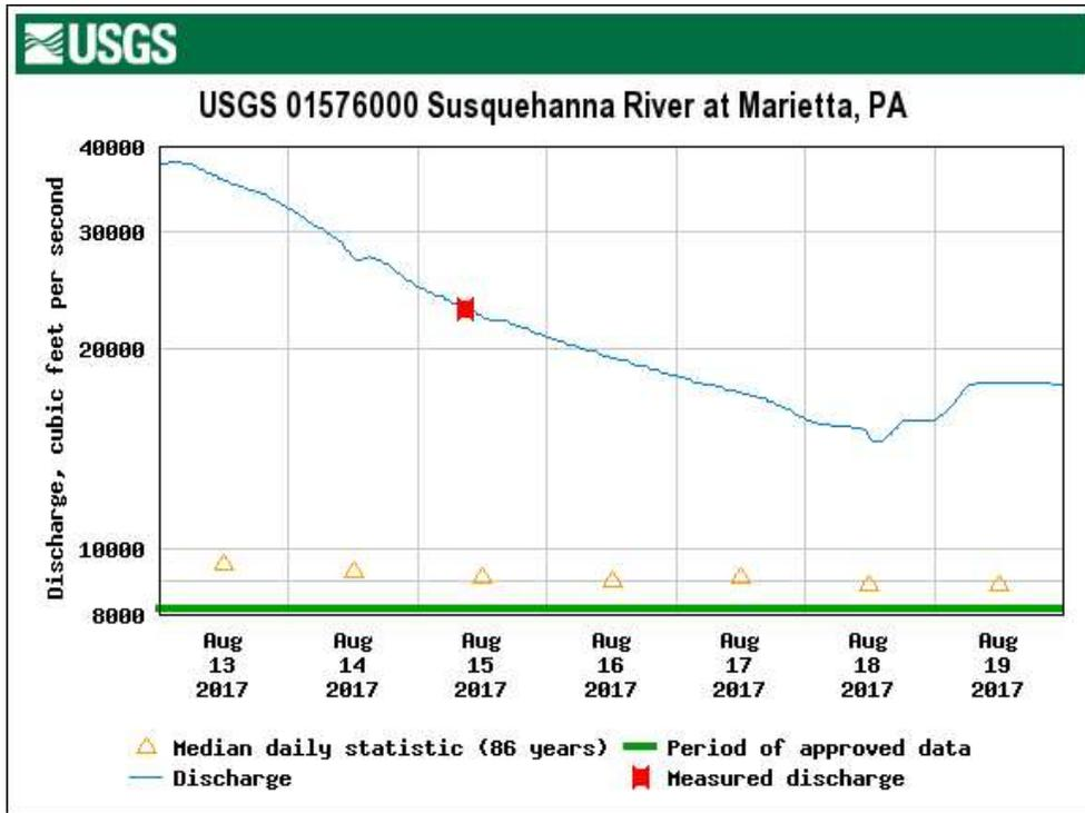
Figure 18: Graph of river discharge (cubic feet per second) at USGS gage 01576000 at Marietta, PA.
