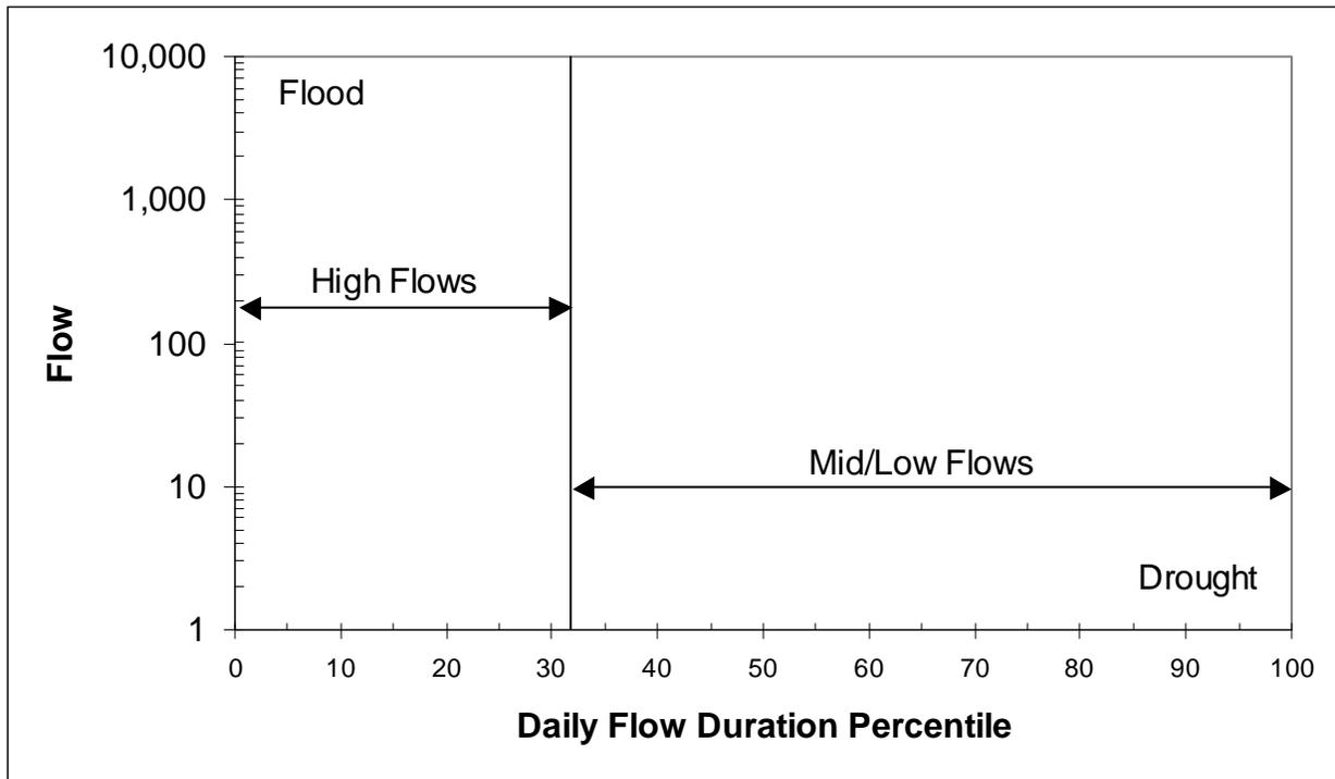
**Figure 2.3.1: Conceptual Diagram of Flow Duration Zones**
