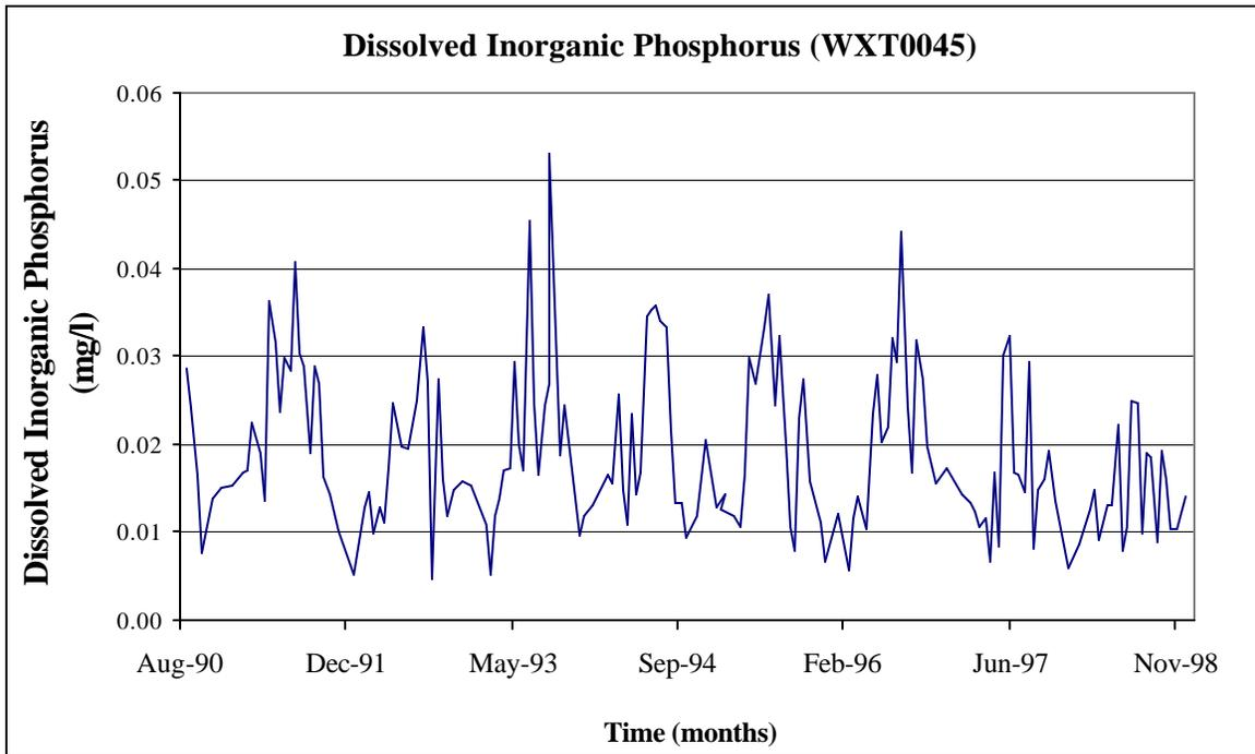
**Figure A6: Dissolved Inorganic Phosphorus Concentrations at Water Quality Station WXT0045**
