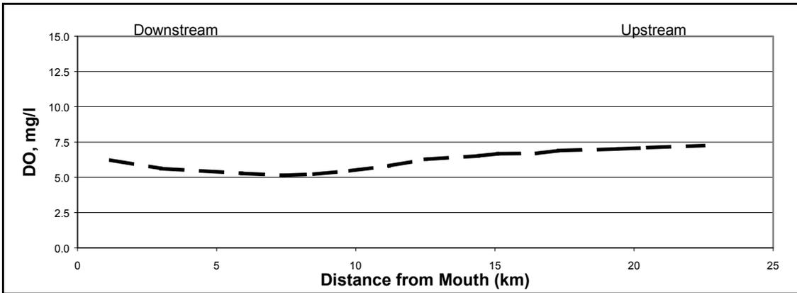
**Figure A27: Dissolved Oxygen vs. River Mile for the Baseline Condition Low Flow Scenario**
