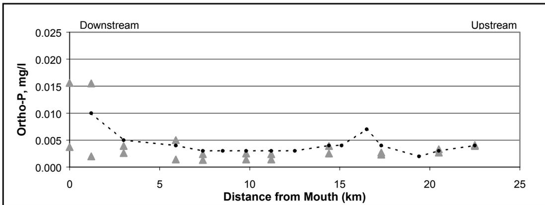
Figure A17: Ortho-Phosphate vs. River Mile for the Calibration of the Model (Low flow)
