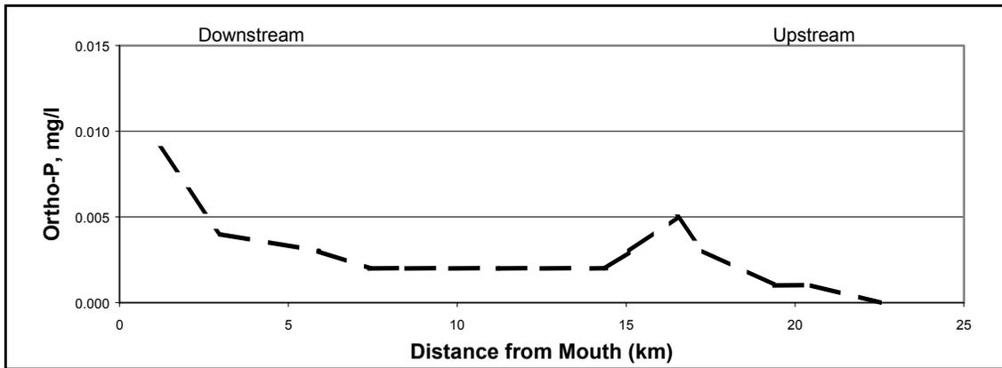
**Figure A33: Ortho-Phosphorus vs. River Mile for the Baseline Condition Low Flow Scenario**
