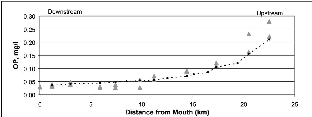
Figure A16: Organic Phosphorus vs. River Mile for the Calibration of the Model (Low flow)
