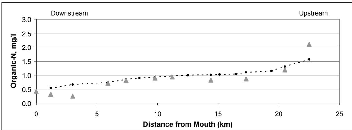
**Figure A22: Organic Nitrogen vs. River Mile for the Calibration of the Model (High flow)**
