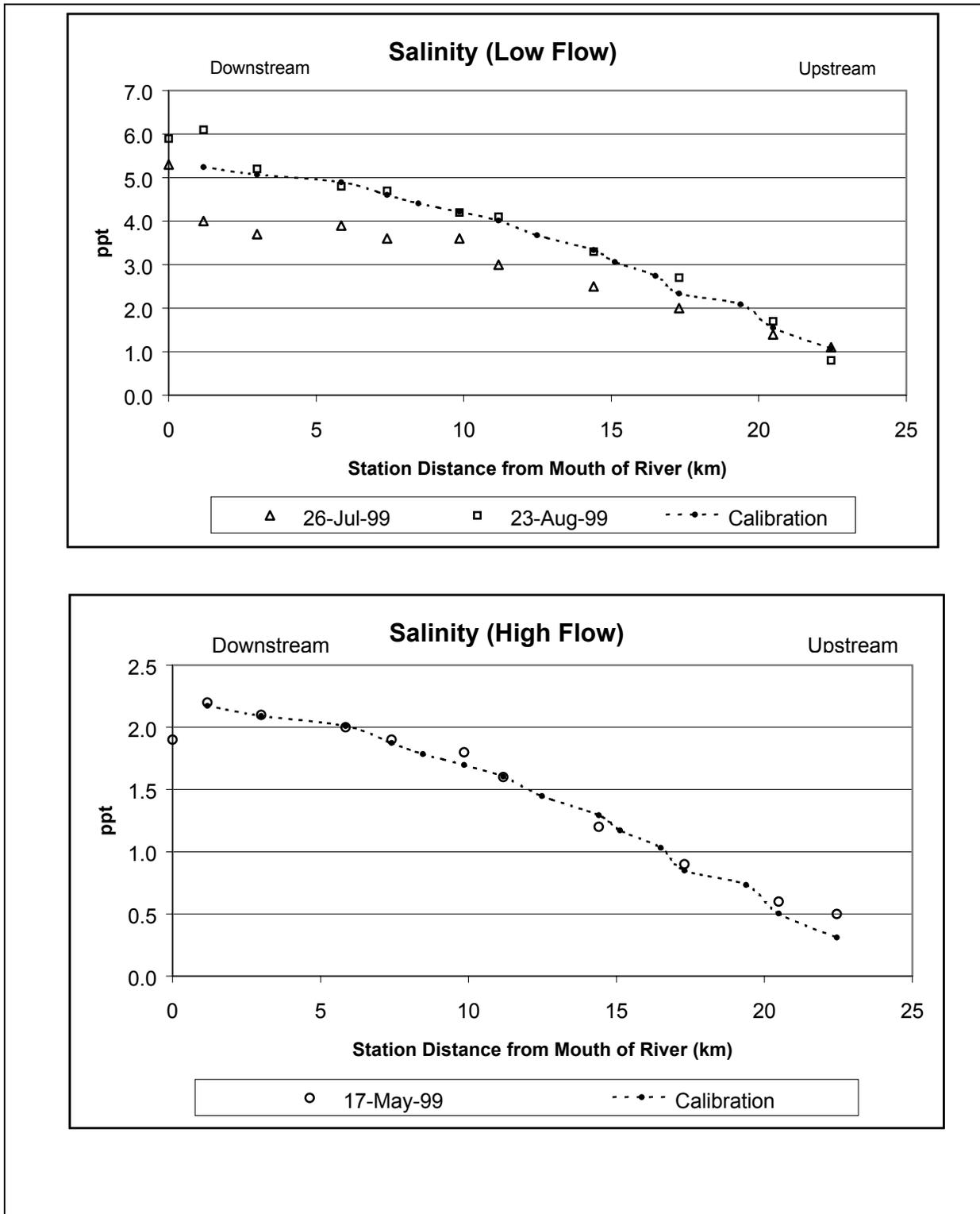
**Figure A8b: Results of Calibration of Exchange Coefficients**
