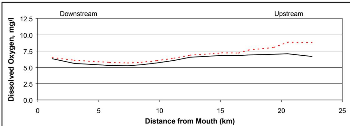
**Figure A51: Dissolved Oxygen vs. River Mile for the Future Average Flow TMDL Scenario**
