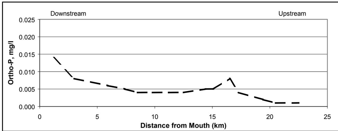
**Figure A41: Ortho-Phosphorus vs. River Mile for the Baseline Condition Average Flow Scenario**
