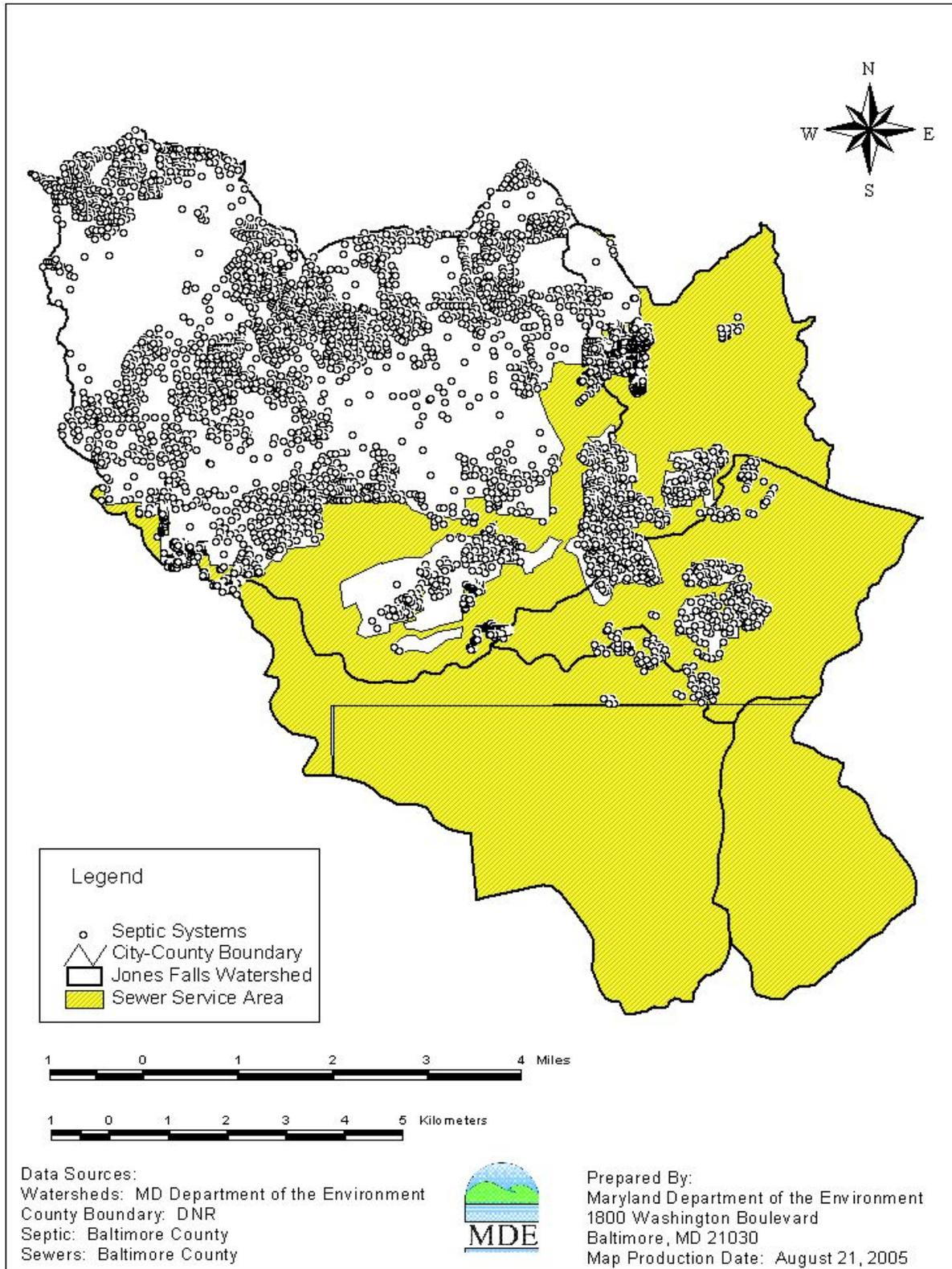
**Figure 2.4.1: Sanitary Sewer Service Area and Septics in the Jones Falls Watershed**
