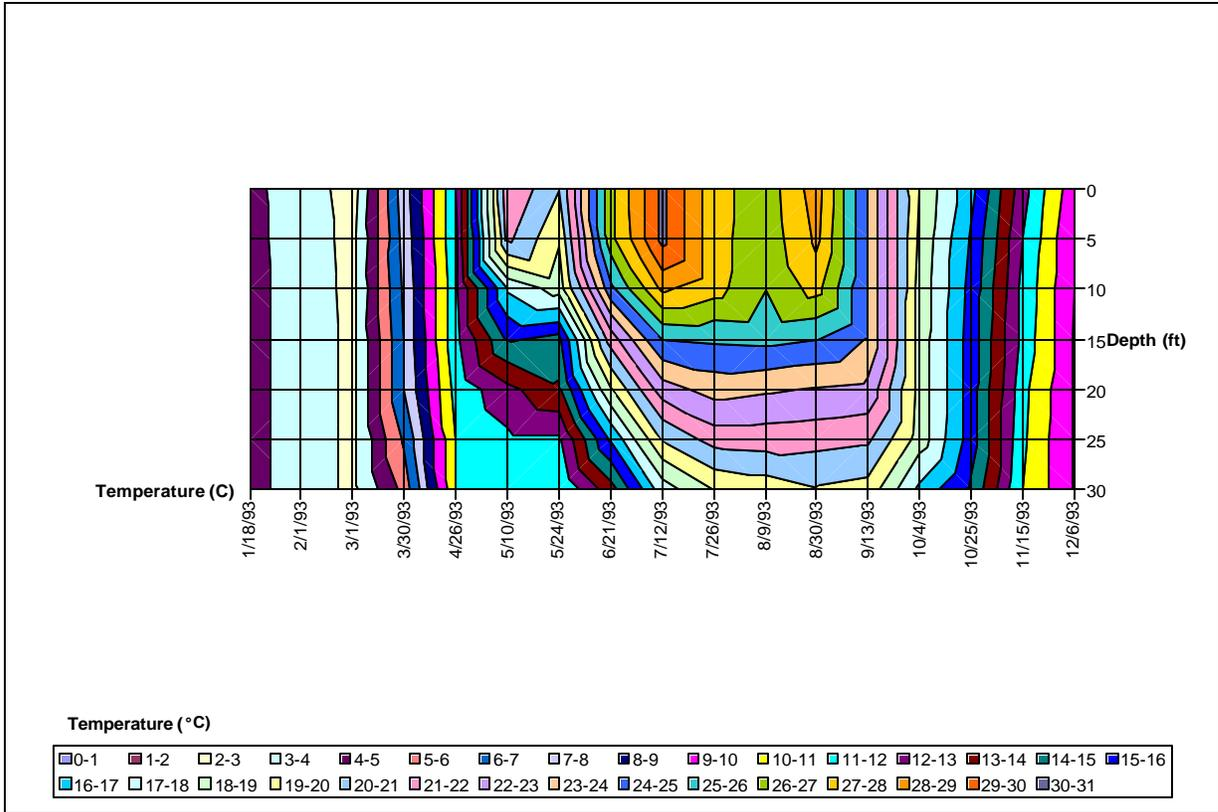
**Figure 10: Isothermal Contours, Loch Raven Reservoir, Middle Stations, 1993**
