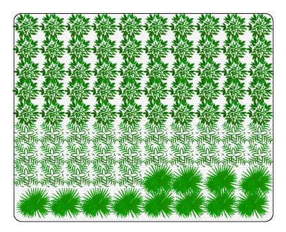
Figure 5. Example illustration of a 500-square-foot bioretention with three species, with the number of plants required to create 85% cover as calculated using Equation 1. Species have been planted in discrete sections but may alternatively be mixed throughout the facility.
