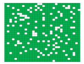
Figure 6. Example of a simple grid that may be used to estimate 85% cover within a best management practice. Green squares represent plant cover, and white squares represent bare or mulched area.
