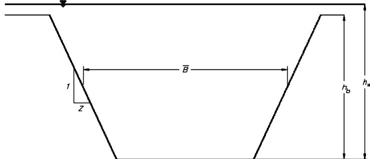
Figure 1. — Parameters of an idealized dam breach.
