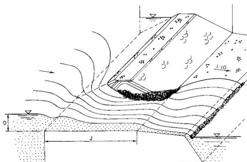
Figure 7. — Lateral erosion of fuse plug embankments (Pugh, 1985).
