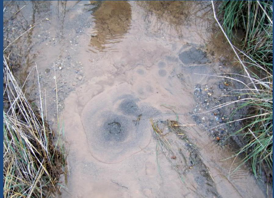
Actively piping sand boil at downstream toe of dam
