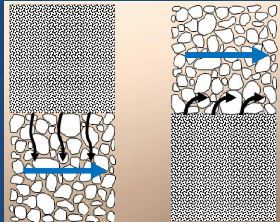
**Figure 26-28. Contact Erosion Process
