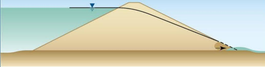
C. Piping progresses backward as particles are detached from exit face. Tunnel forms.
