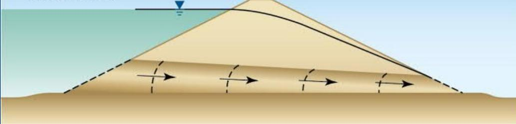
D. Reservoir empties through tunnel, breach occurs. Tunnel may collapse if wide enough.
