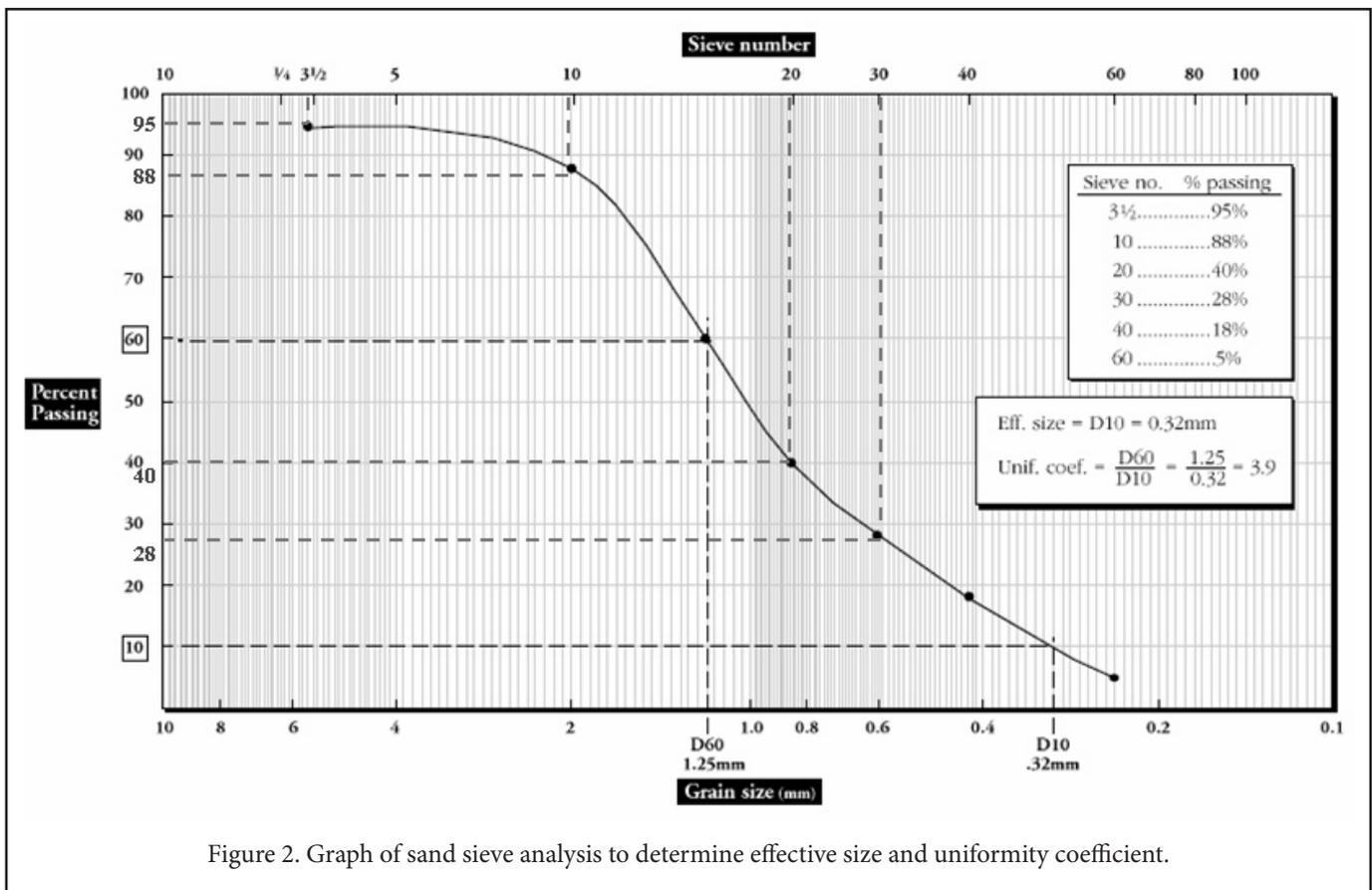
Figure 2. Graph of sand sieve analysis to determine effective size and uniformity coefficient.
