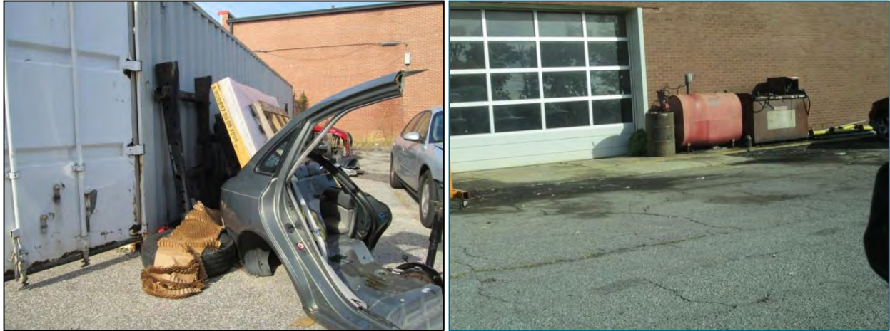
Figure 4-12: Potential Pollution Sources from Outdoor Material Storage at Auto-related Hotspots including uncovered materials stored outside (left) and storage containers without secondary containment (right).
