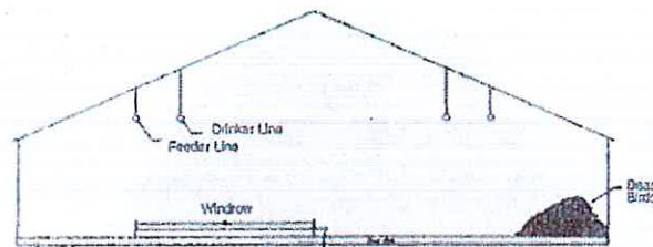
Figure 3. Create a windrow 12 feet wide with a base on one side of the house. Make sure outer edge of the windrow does not go beyond feeder line boundary.
