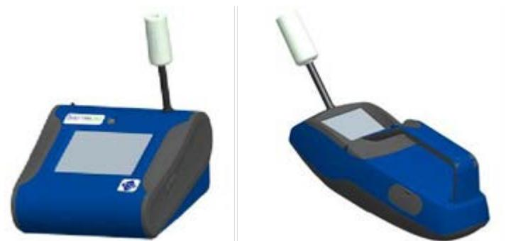
Run **Zero Cal** prior to every 24-hour sampling event. Zero Cal requires that the zero filter be attached prior to running. Zero Cal must also be performed if the unit is reading negative concentrations. It is not possible for the DustTrak monitor to read negative concentrations. Negative concentrations are a symptom of zero drift.
