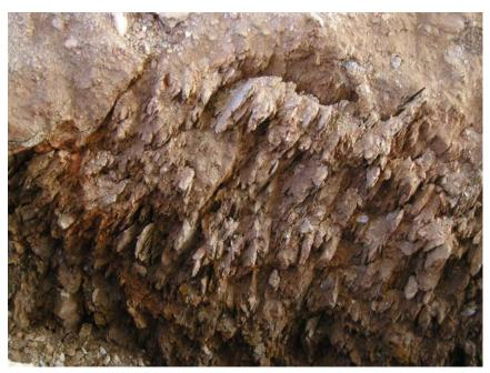
Photo 2-A close-up view of folded relict bedding planes (dip East) observed during excavation under the canopy approximately 5 to 8 feet below ground surface in the weathered phyllite. The view is towards North with the station building behind the viewer.
