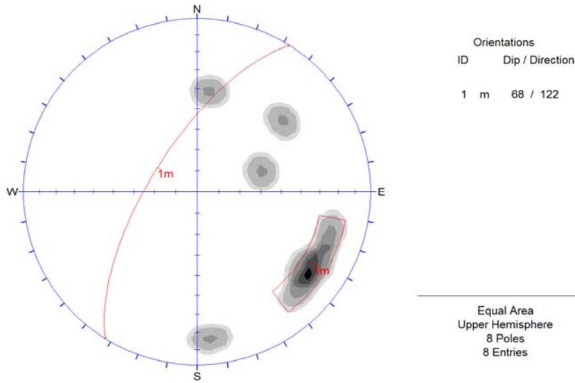
Figure 5: Polar diagram with statistical contouring of bedding planes set. Calculated mean dip angle and direction is shown at the right of the diagram.
