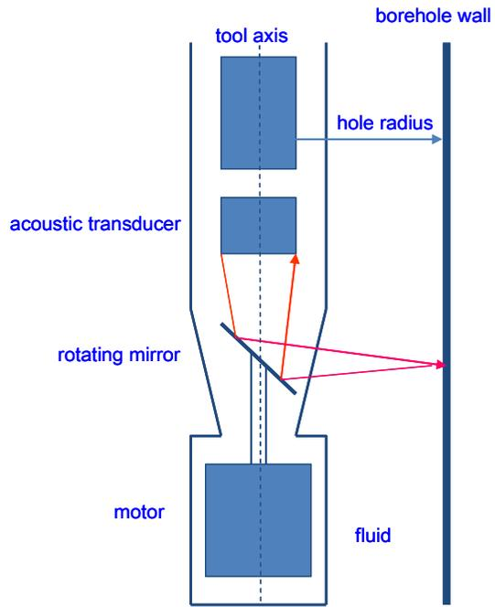
Figure A- 6: Schematic of the acoustic televiewer tool.
