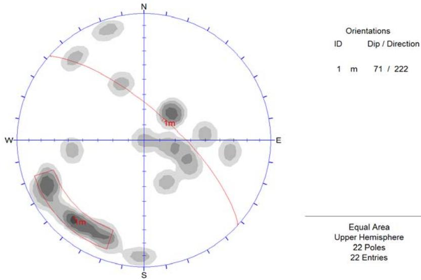
Figure 7: Polar diagram with statistical contouring showing mean orientations of fractures sets. The calculated mean of each set is shown at the right of the diagram.
