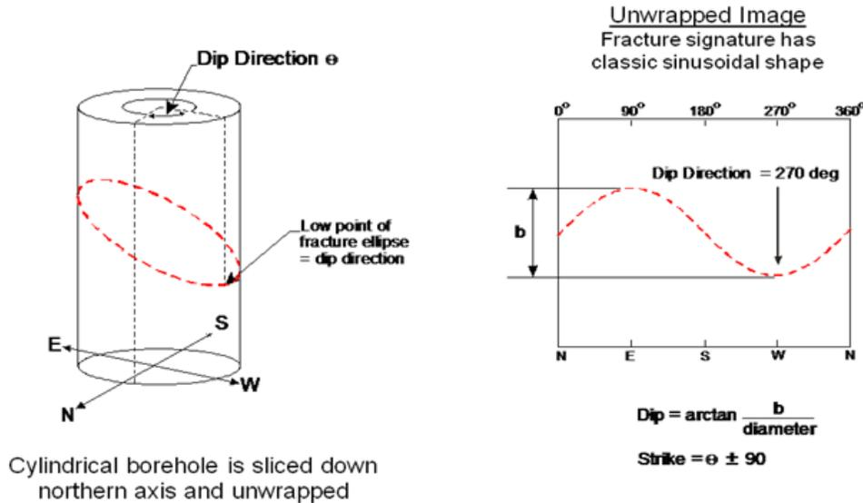
Figure A- 5: Schematic showing the sinusoidal fracture signature in the unwrapped borehole view.
