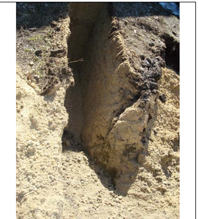
Photo 8: Test pit with gasoline-contaminated soils, adjacent to UST Target #'s 8 and 9.
