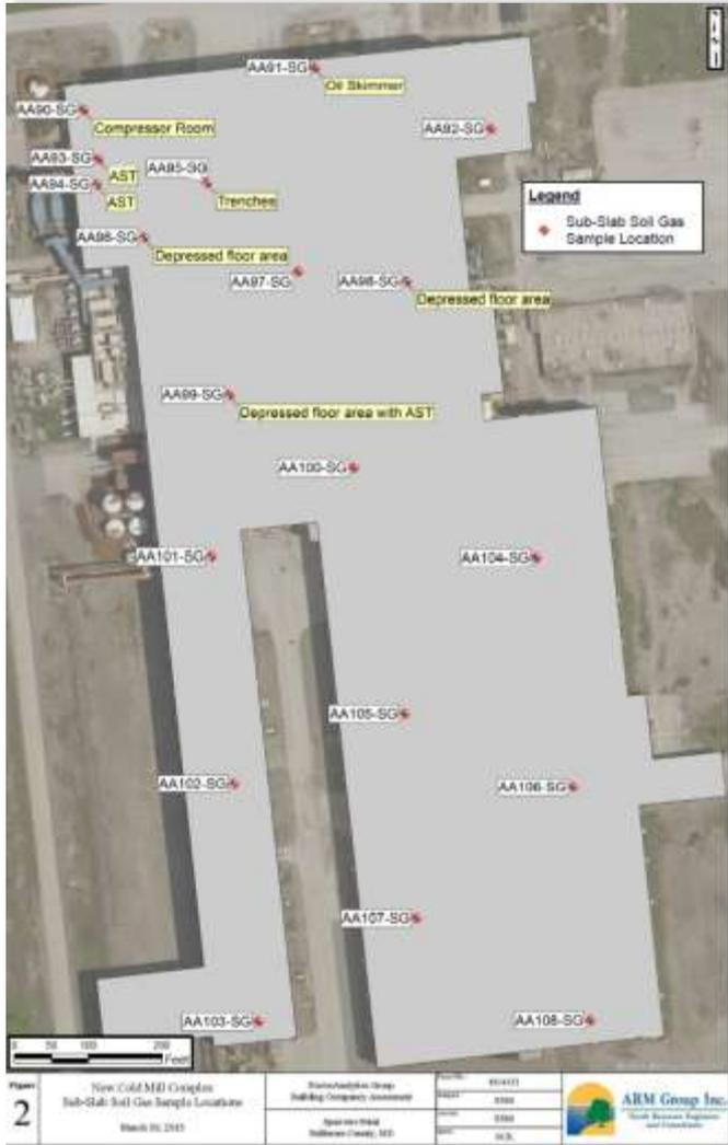
April 2015 Occupancy Assessment to evaluate sub-slab soil gas conditions. 19 Sub-slab Soil Gas Sampling Locations. No elevated levels of soil vapor contaminants were detected above MDE Tier 1 Screening Levels
