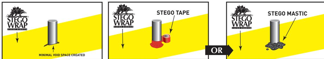
**STEGO WRAP PIPE PENETRATION REPAIR DETAIL:**
