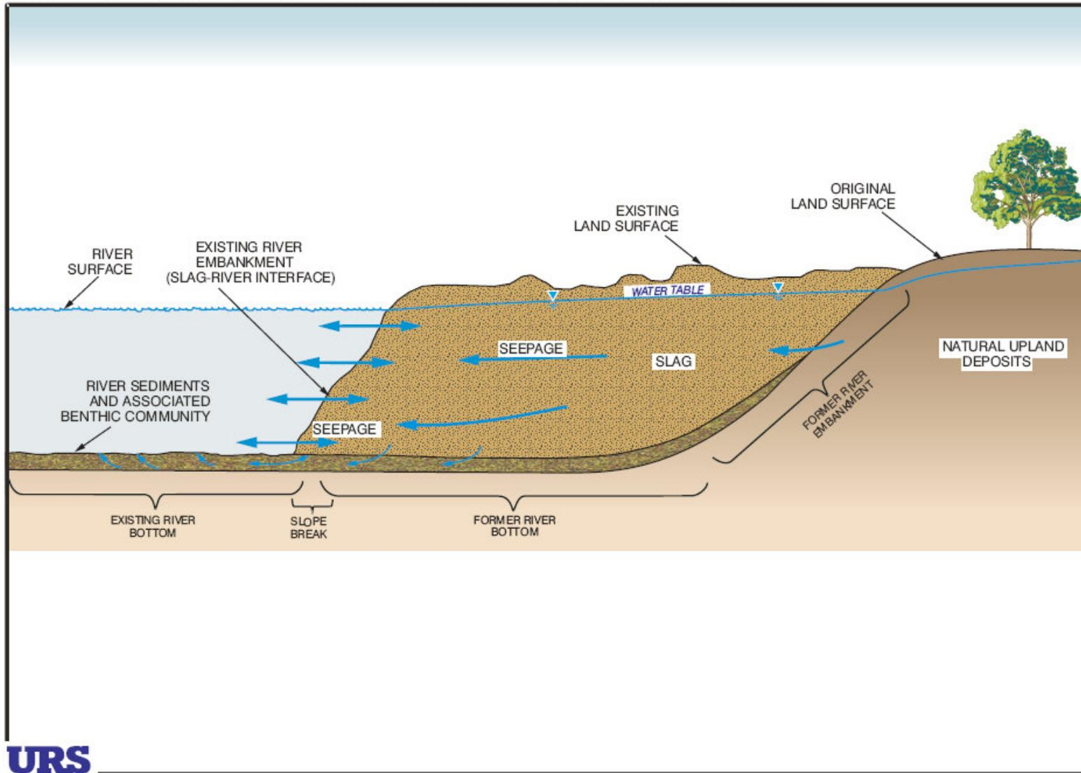
Figure 5. Conceptual Groundwater to Surface Water Flow Model.
