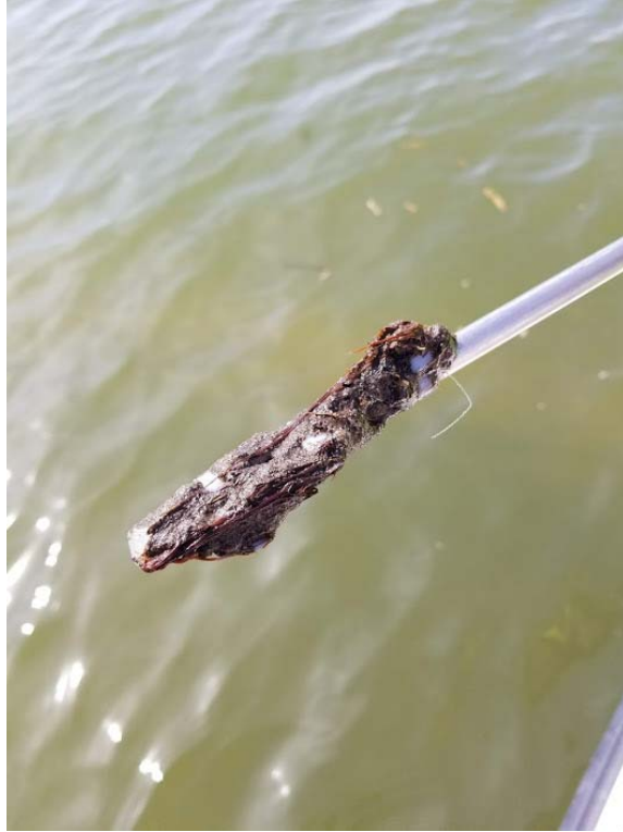
Photo 1: View of RW-013-PW-1 after attempting a 9 inch sample in the Rod and Wire Mill area. Black mud can be observed on the screen filter.
