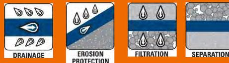
Mirafi® 140N is a nonwoven geotextile composed of polypropylene fibers, which are formed into a stable network such that the fibers retain their relative position. Mirafi® 140N is inert to biological degradation and resists naturally encountered chemicals, alkalis, and acids. Mirafi® 140N meets AASHTO M288 Class 3 for Elongation > 50%.
