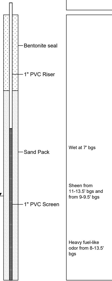
Boring terminated at 14' bgs due to refusal and piezometer installation
