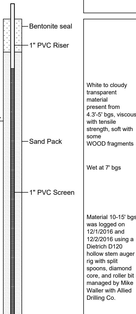
Boring terminated at 20' bgs due to water and piezometer installation
