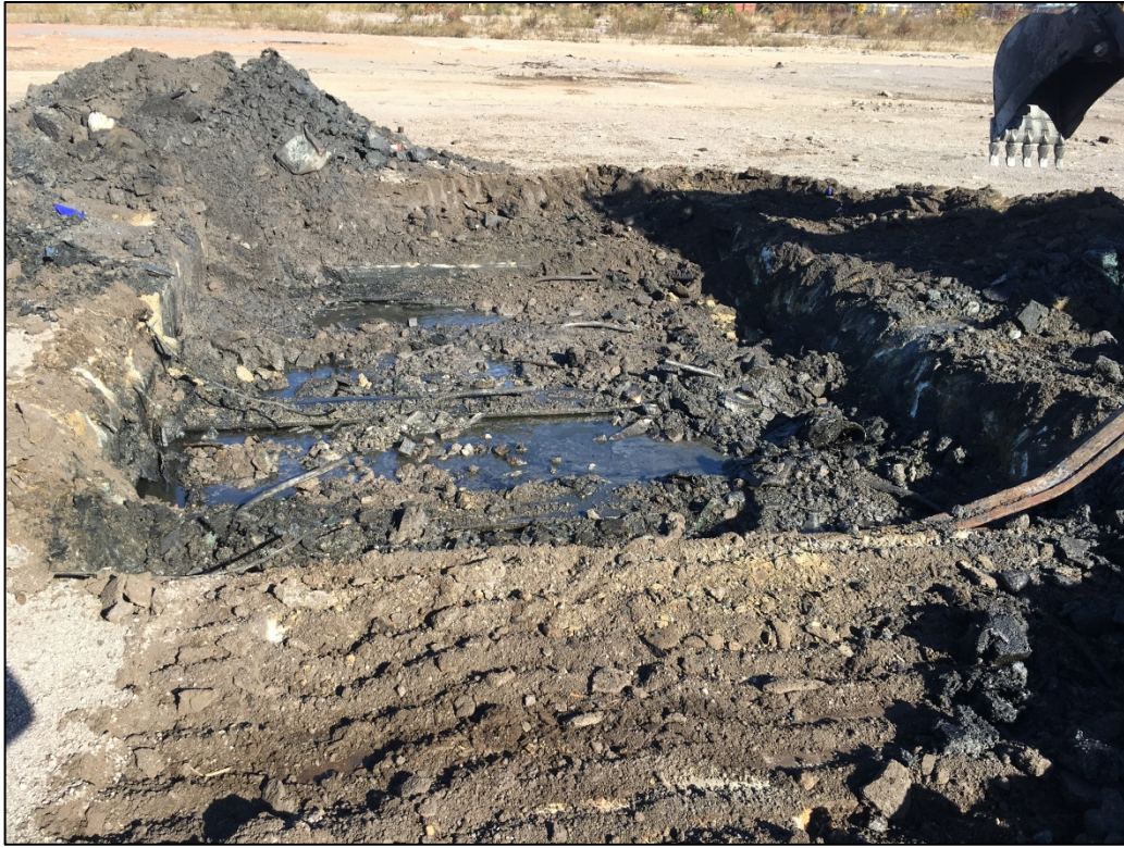
Photo 1: View of test pit at B17-007-SB, facing north, prior to clearing and cleaning. NAPL can be observed on the water.
