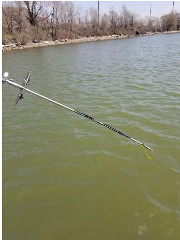
Photo 4: View of CO-045-PW-3 after attempting a 3 foot sample in Cell 3 of the Coke Oven Area. Black mud extends nearly up to the flange of the push-point sampler.
