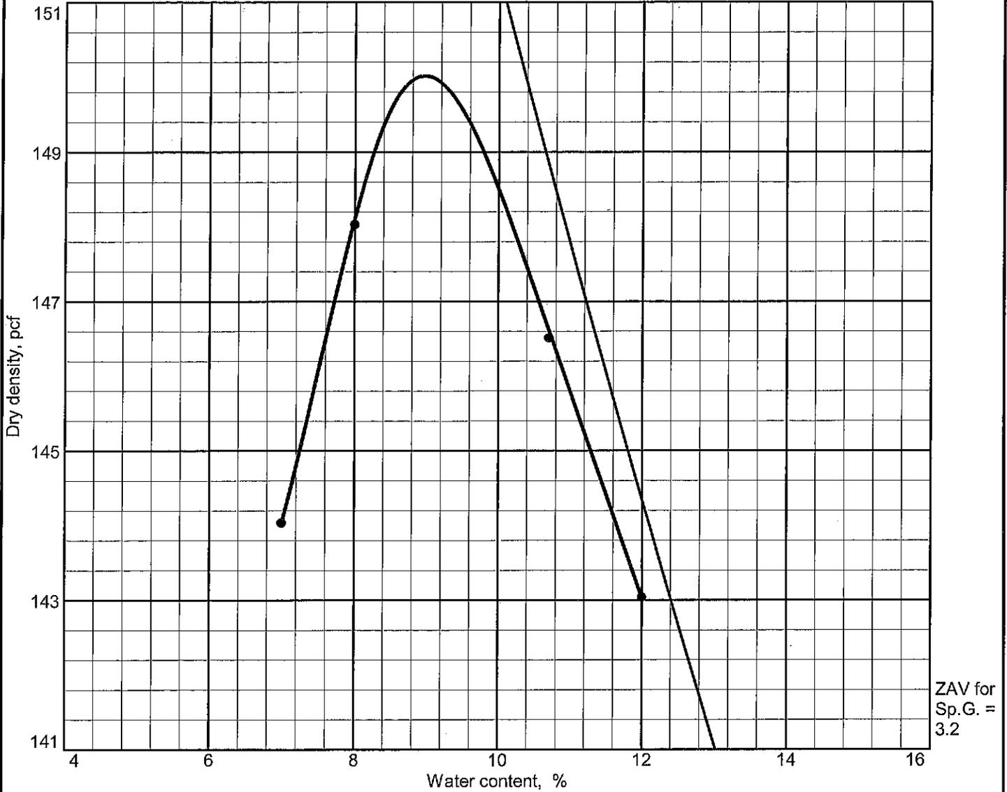
Test specification: AASHTO T 180 Method A Modified
