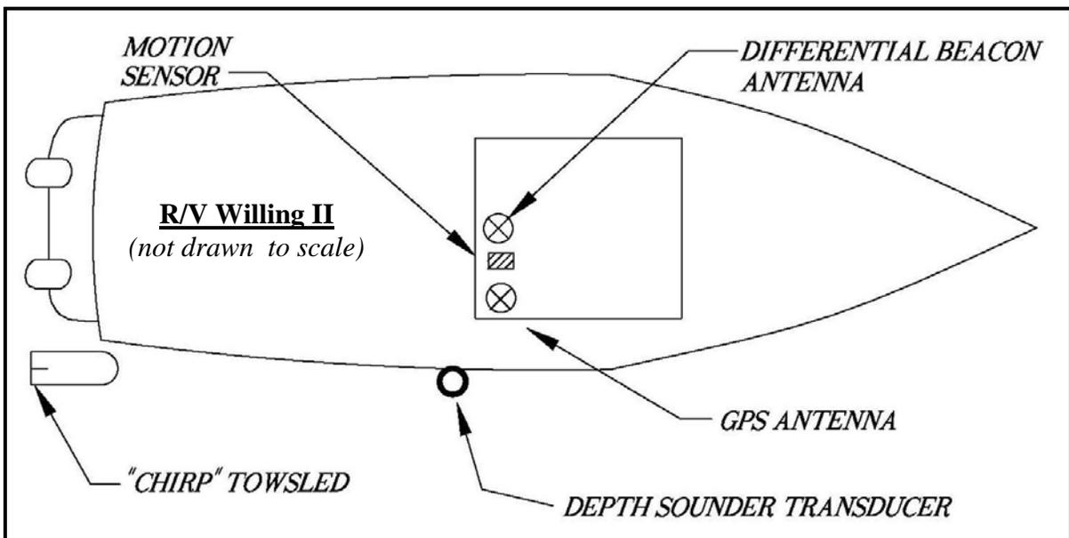
Figure 2. Schematic of instrument configuration during onsite operations.
