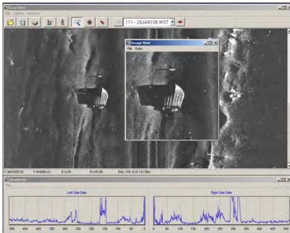
**Side Scan Sonar (SSS) Support:** HYPACK® provides support of SSS systems in its basic package. All analog and several digital side scan systems can be utilized with the SIDE SCAN SURVEY program. Users can display the real time data and perform targeting in real time or post-processing. A program that generates side scan mosaics in Geo-TIF format allows you to plot your results in HYPACK® or export them to your GIS.
