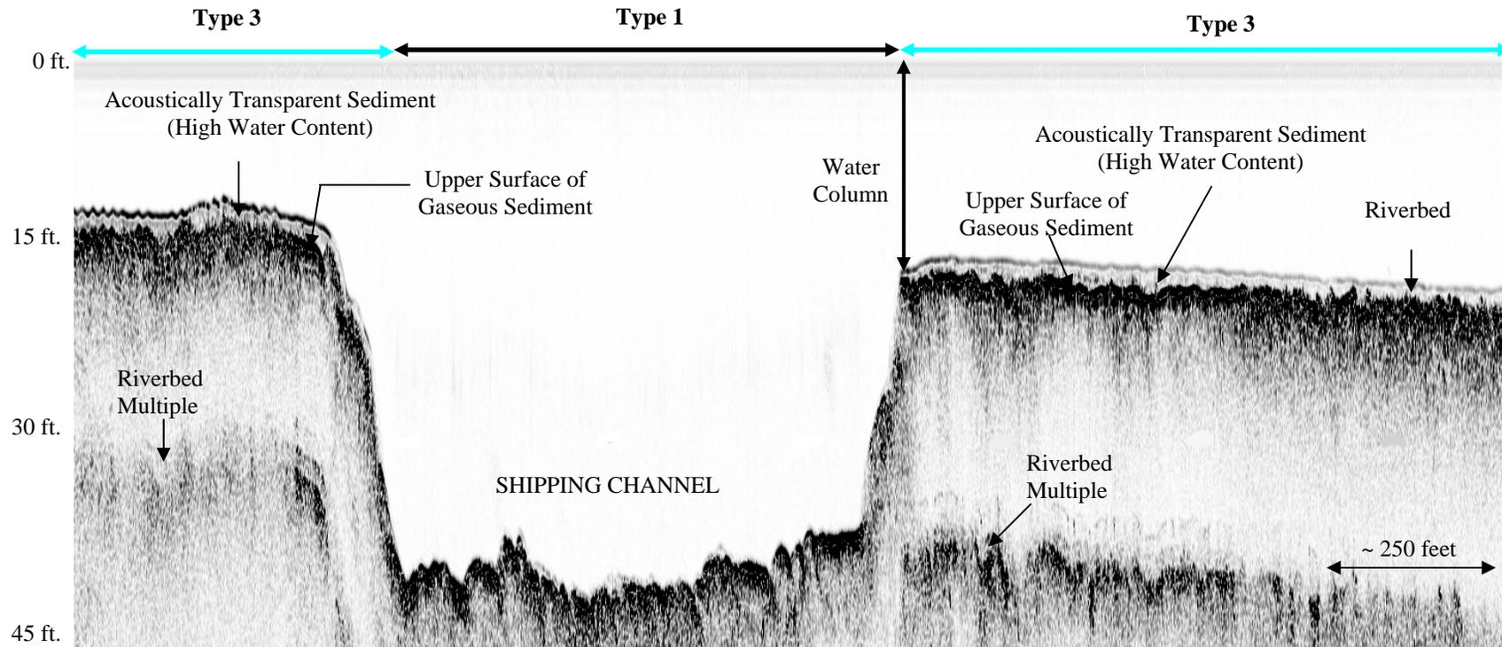
Figure 6: Reproduced section of chirp profile record depicting subbottom data classification Types 1 and 3. Note the thin layer (~2-3') of acoustically transparent sediments that blanket the riverbed in Type 3 areas. The acoustically transparent sediments are generally associated with highly aqueous silts.
