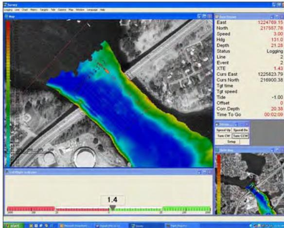
**SURVEY:** HYPACK® contains interface drivers to over 200 devices including positioning systems, echosounders, heave-pitch-roll sensors, gyros and other types of equipment. SURVEY supports a single vessel or multiple vessels, along with towfish and ROVs. Data is logged with incredible precision (<1mSec). Survey data and windows can be broadcast over a network to any other computer or saved to a file using our Shared Memory Output routines.
