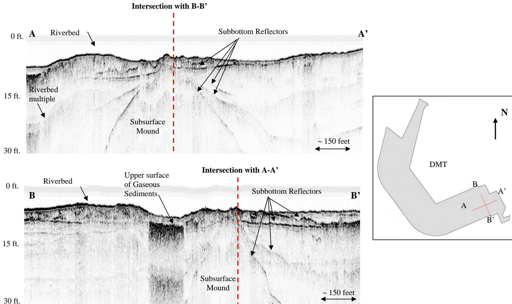
Figure 9: Reproduced sections of chirp subbottom profile records depicting unusual subsurface mound identified in the southeastern margin of site. Sections of two orthogonal profiles intersecting at the apex of several steeply dipping subbottom reflectors illustrate the asymmetry of an unusual subbottom feature. Location map illustrates the position of each profile in the survey area. The images have an approximate vertical exaggeration of 16:1.
