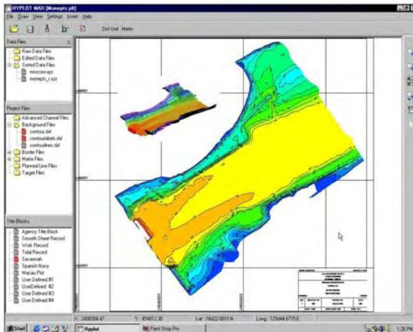
**FINAL PRODUCTS:** The ability to create the final products you need separates HYPACK® from the rest. The plotting program generates professional smooth sheets with soundings, grids, graphics and contours in a WYSIWYG display. The VOLUMES program is the de facto standard of the U.S. Army Corps of Engineers for the computation of quantities in dredging projects. TIN MODEL creates surface models that can be used for contouring, volume computations and surface visualization.
