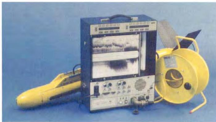
The EPC Model MP-1086 is a multi-purpose recording system that serves as a continuous gray scale printer, analog tow fish interface, mass storage device, and signal processor.
