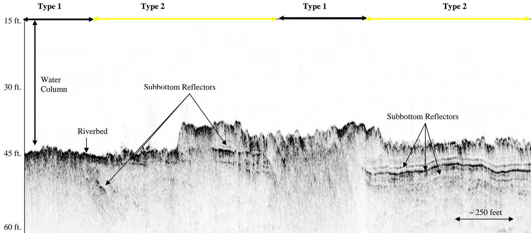
Figure 5: Reproduced section of chirp profile record depicting subbottom data classification Types 1 and 2. These profile categories are representative of the shipping channels. Type 1 refers to areas where no subbottom penetration was observed. Type 2 refers to areas of generally horizontal and closely spaced reflectors that terminate abruptly.
