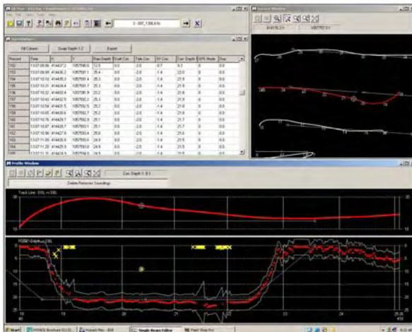
**EDITING:** The SINGLE BEAM EDITOR program is used to quickly review your survey data and to automatically and/or manually remove outliers. Sounding data is simultaneously displayed in plan, spreadsheet, and profile views with the channel design info drawn in the backgrounds. Routines developed by HYPACK® from collaboration with the U.S. Army Corps of Engineers to integrate water level corrections based on RTK GPS elevation info are a standard part of package.
