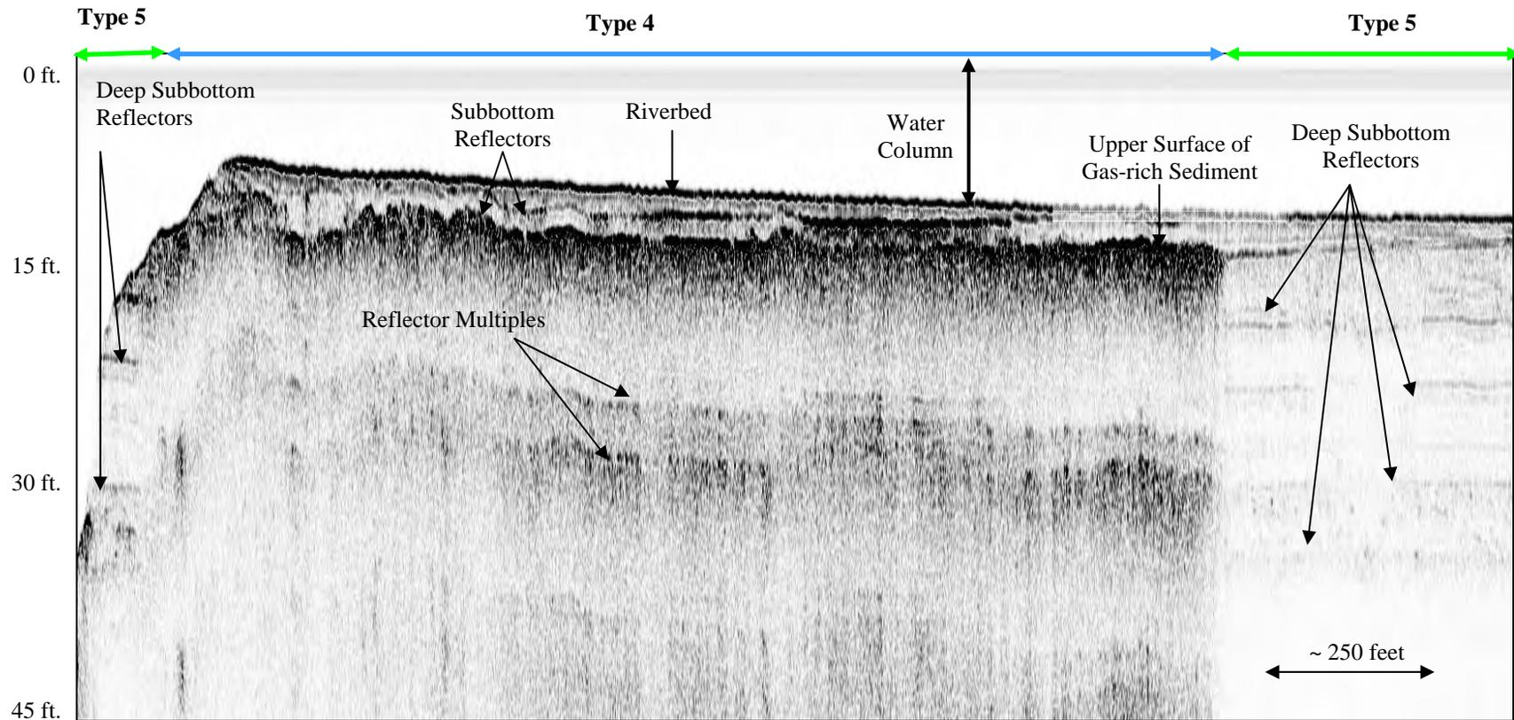
Figure 7: Reproduced section of chirp profile record depicting subbottom classification Types 4 and 5. Type 4 is characterized by a minimum of one subbottom reflector, which generally overlies a gas-rich sediment horizon. Type 5 is associated with deep subbottom penetration and the detection of multiple subbottom reflectors. Note the abrupt transition from Type 4 to Type 5 and the lack of deep subbottom reflectors in the Type 4 data.
