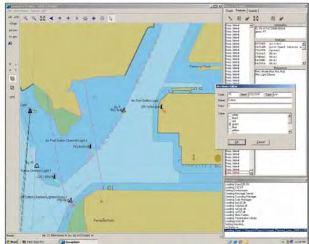
**ENCEdit** is a new HYPACK® module that allows you to create, modify and verify ENC data in S-57 format. ENCEdit provides you with tools to re-attribute, create, move or delete existing features. You can also create new features by manually entering coordinates, by importing data from DXF/DGN, or by transferring targets in real time from SURVEY directly into ENCEdit.
