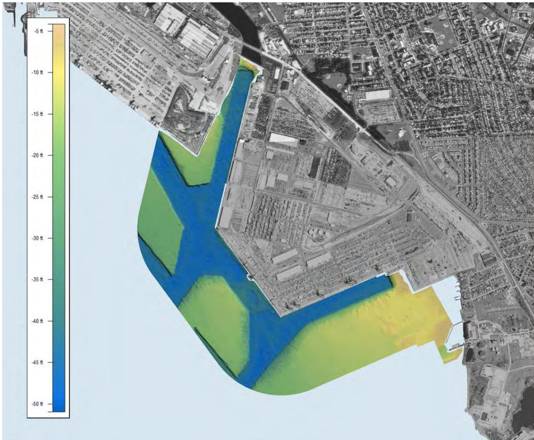
Figure 4: Hydrographic data presented in plan view using color to represent depth (vertical datum: NAVD88).
