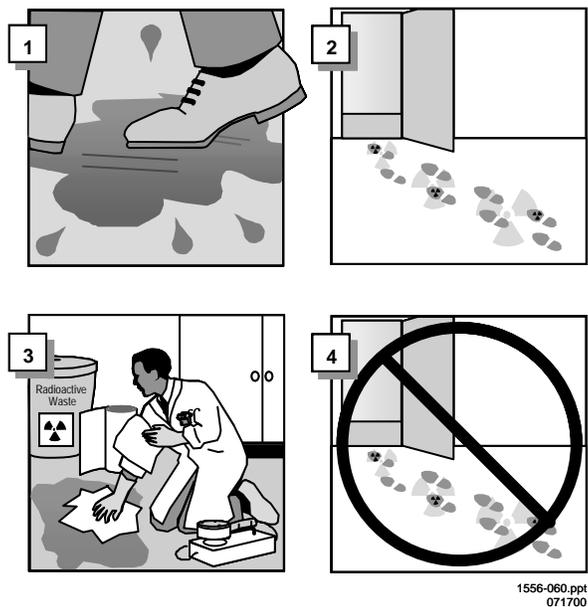
**Figure 8.14 Proper Handling of Incident.** *Panels 1 and 2 indicate how contamination can be spread if the incident is not handled properly as in panels 3 and 4.*
