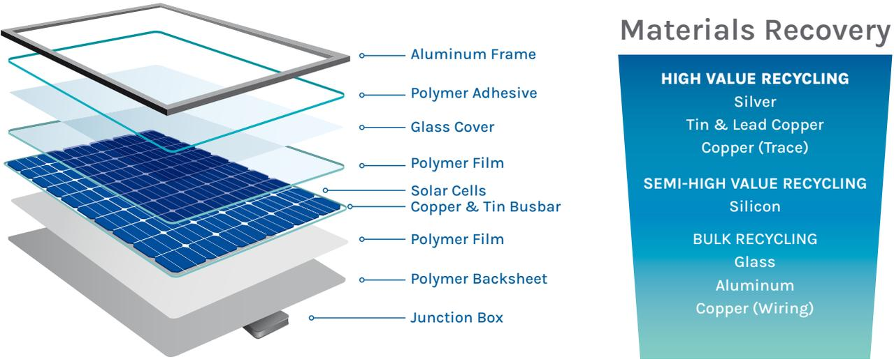
**Figure 5.** Schematic of solar panel materials and which materials are captured in different types of recycling processes. The materials are divided into categories according to their value after recycling.
