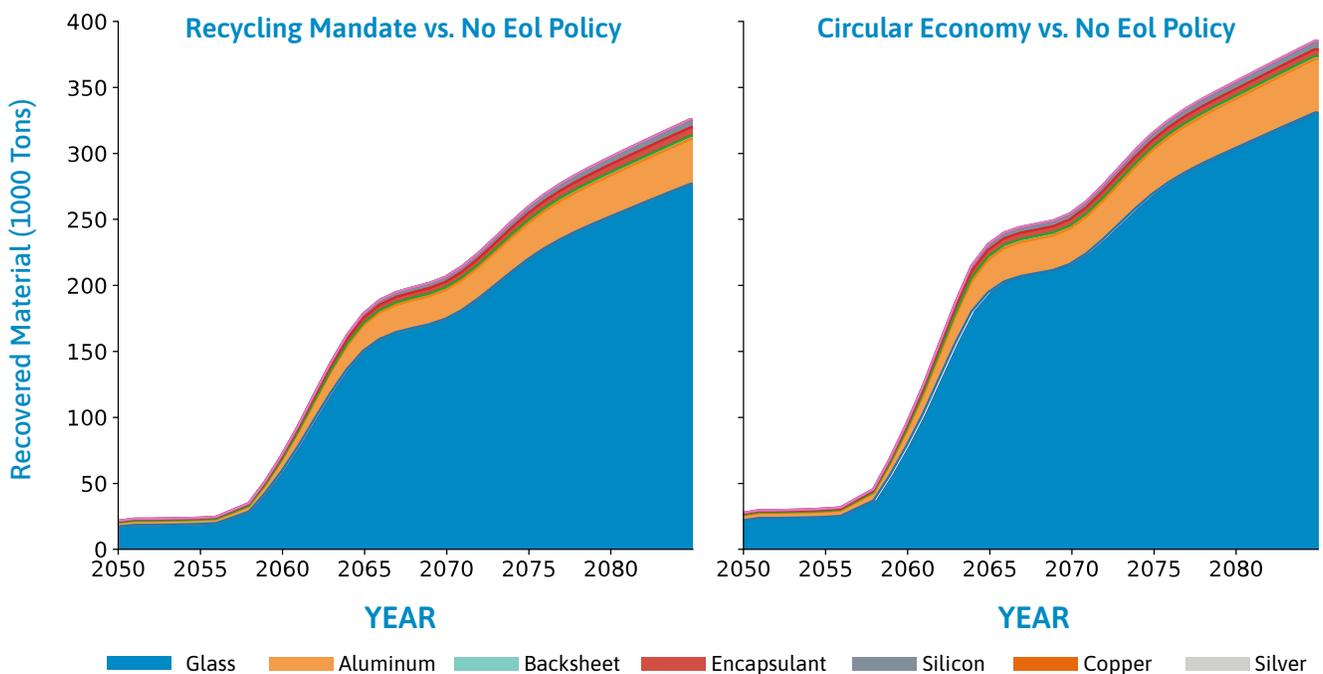
**Figure 10.** (b) The recovered material that is returned to the supply chain if either a recycling mandate or a circular economy EoL management policy is adopted (as compared to landfilling).
