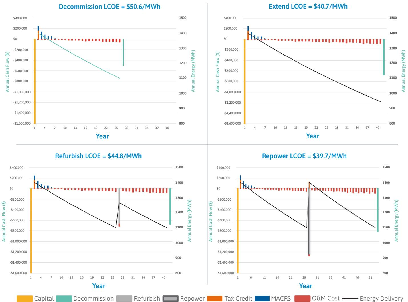
**Figure 2.** Representative cases of cash flow analysis based on different end-of-life options. Financial model developed by National Renewable Energy Laboratory (NREL) and updated by the authors.<sup>12</sup> Note that this only includes a few revenue sources, and it does not include revenue from selling energy generated. O&M = Operations and Maintenance. MACRS = Modified Accelerated Cost Recovery System, a method of depreciation. Further details are provided in the technical appendix.
