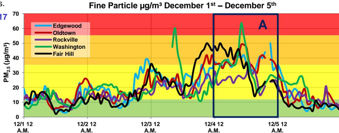
Figure 4: PM<sub>2.5</sub> concentrations (µg/m<sup>3</sup>) for several monitors between the timeframe of December 1<sup>st</sup> – December 5<sup>th</sup> 2017. Horizontal coloring matches with appropriate AQI ranges. December 1<sup>st</sup> – 3<sup>rd</sup> shows the gradual increase in PM<sub>2.5</sub> concentrations leading up to the exceedance event on the 4<sup>th</sup> marked by the blue box labeled "A".
