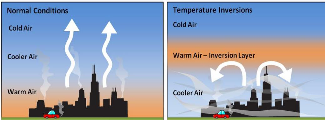
*Figure 3: Conceptual comparison showing pollutant impacts under “normal conditions” (decrease in temperature with height) and temperature inversions (increase in temperature with height).*
