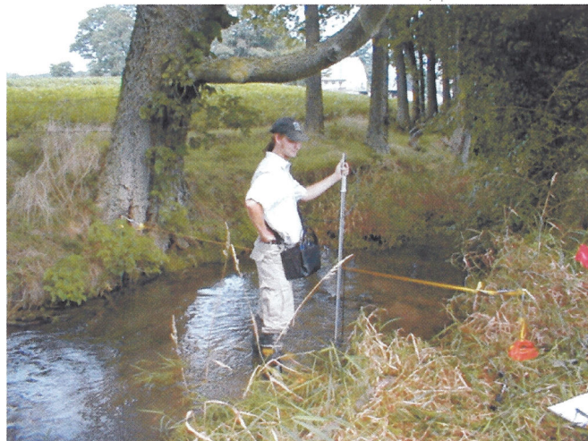
Measuring discharge on the tributary to St James Run at stream gaging site 1.
