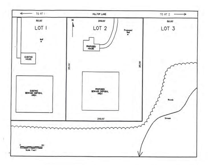
FIGURE 3.2 Example site plan.
