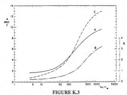
Dimensionless parameters A, B, and C as a function of  $L_e/r_W$  for calculation of  $\ln(R_e/r_W)$ .
